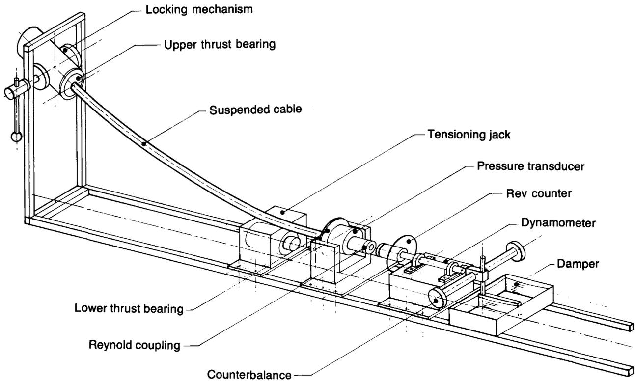
Fig. 4—Isometric sketch of the layout of the test apparatus
