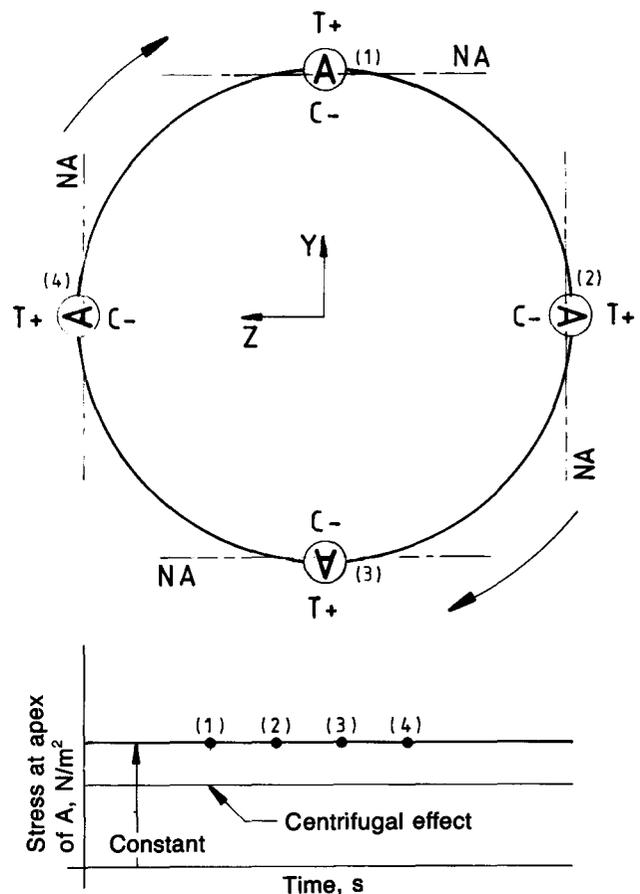
Fig. 2—Flexure stress occurring at a fixed point on the cable, rotational motion
