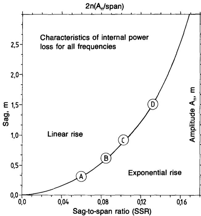
Fig. 9—Loci of critical sag-to-span ratios
