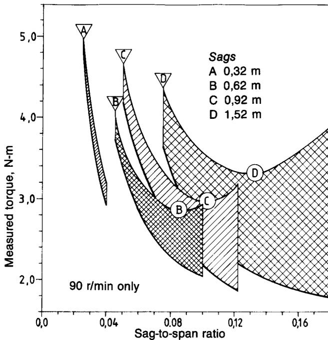
Fig. 7—Energy levels (the upper traces indicate total measured torque, and the lower traces indicate bearing loss)
