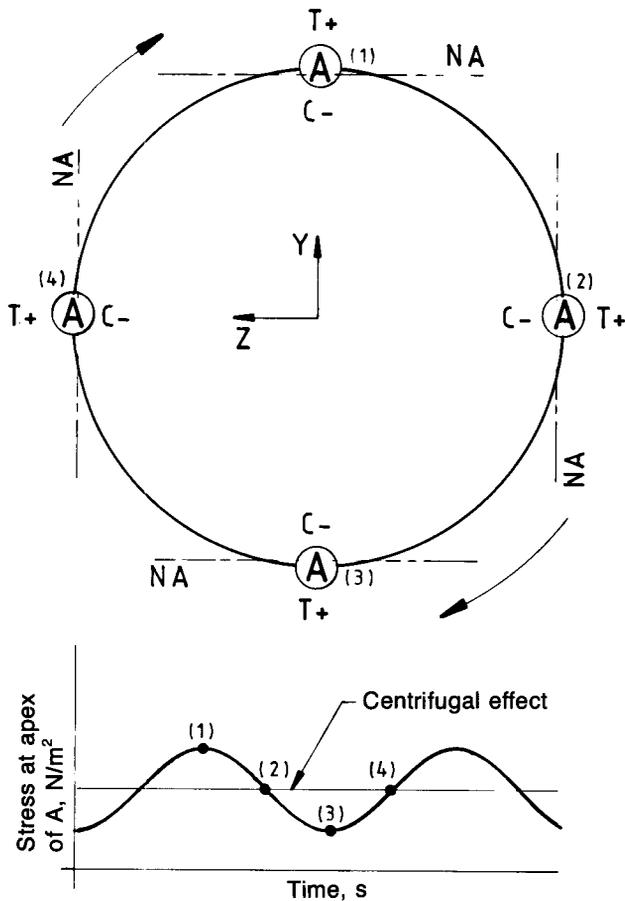
Fig. 3—Flexure stress occurring at a fixed point on the cable, irrotational motion
