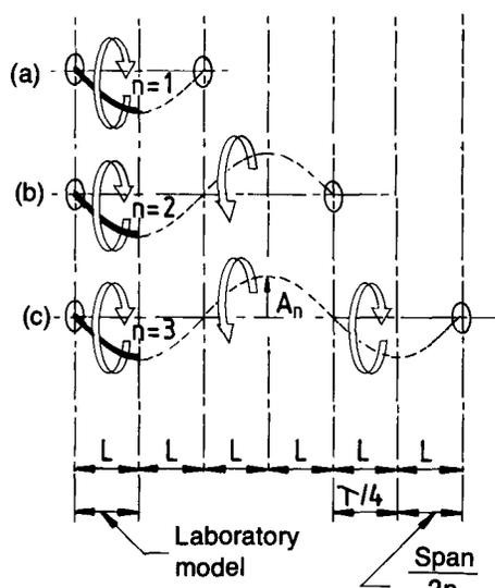
Fig. 10—Higher modes of harmonic vibration
