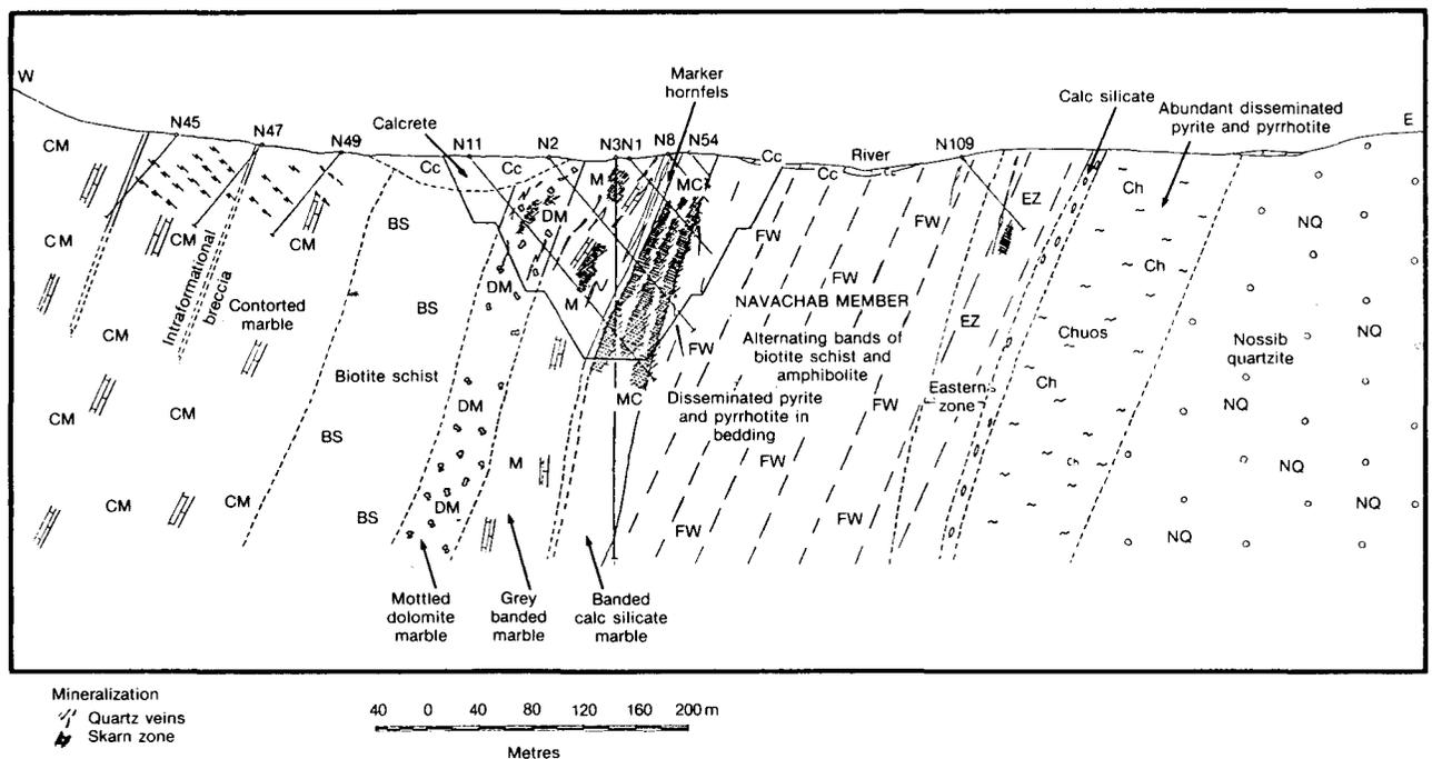
Fig. 2—A geological section at the Navachab Mine as interpreted from borehole sections and surface mapping
