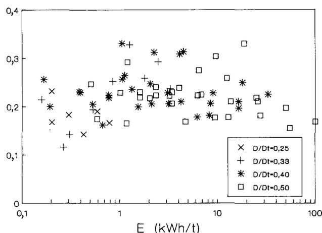
Fig. 2—Klimpel parameters for  $U_3O_8$  and gangue as a function of conditioning energy (pitched-blade impeller at standard geometry, ore A)
