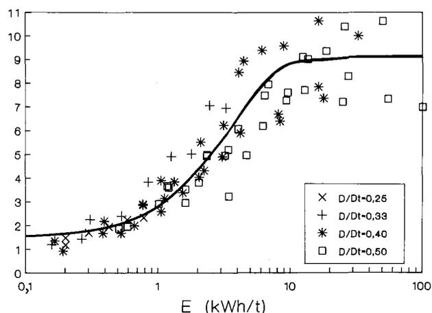
Fig. 1—Klimpel parameters for gold and sulphur as a function of conditioning energy (pitched-blade Impeller at standard geometry, ore A)
