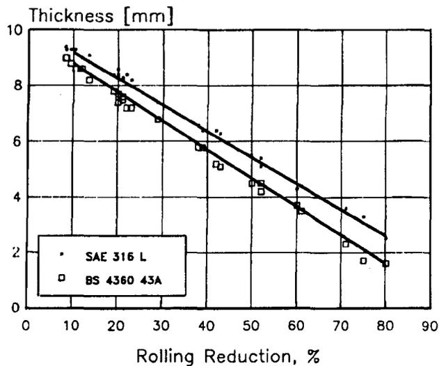
Fig. 5—Comparison of the reduction in thickness of carbon and stainless steels
