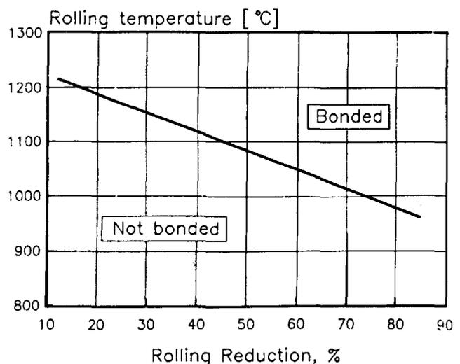
Fig. 7—Threshold deformation in relation to rolling temperature
