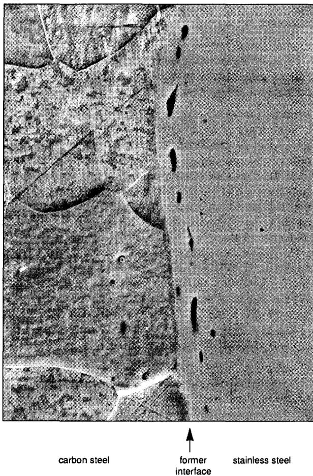
Fig. 6—Dispersed and partly dissolved oxides in the former interface between a stainless and a carbon steel (SEM, original magnification 2000 X)
