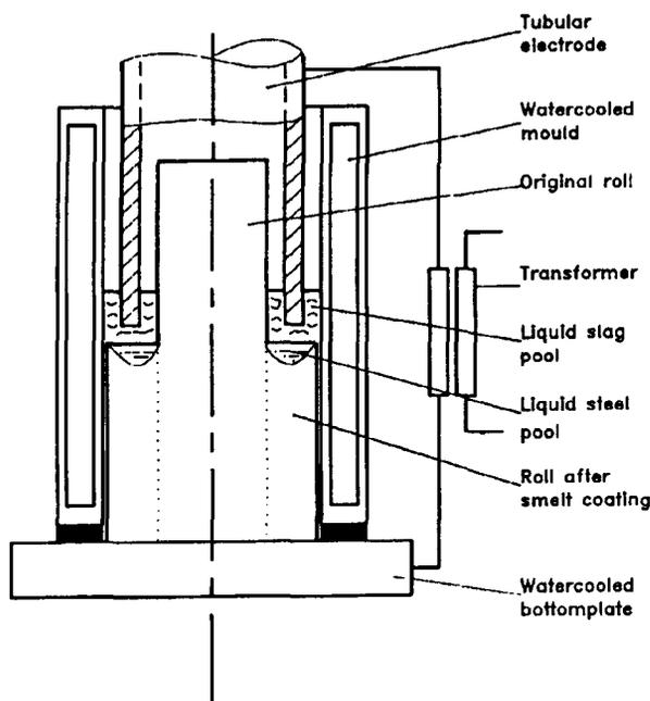
Fig. 1—Building up of a roll by the electro-slag remelting process
