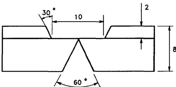
Fig. 3—Example of groove preparation for butt welding
