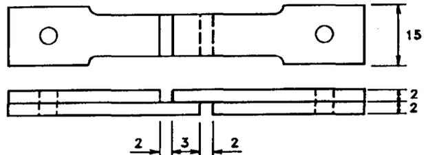
Fig. 4—Schematic representation of a sample used in the determination of bonding strength
