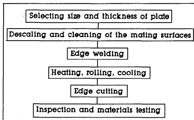
Fig. 2—Flowsheet for the manufacture of flat products
