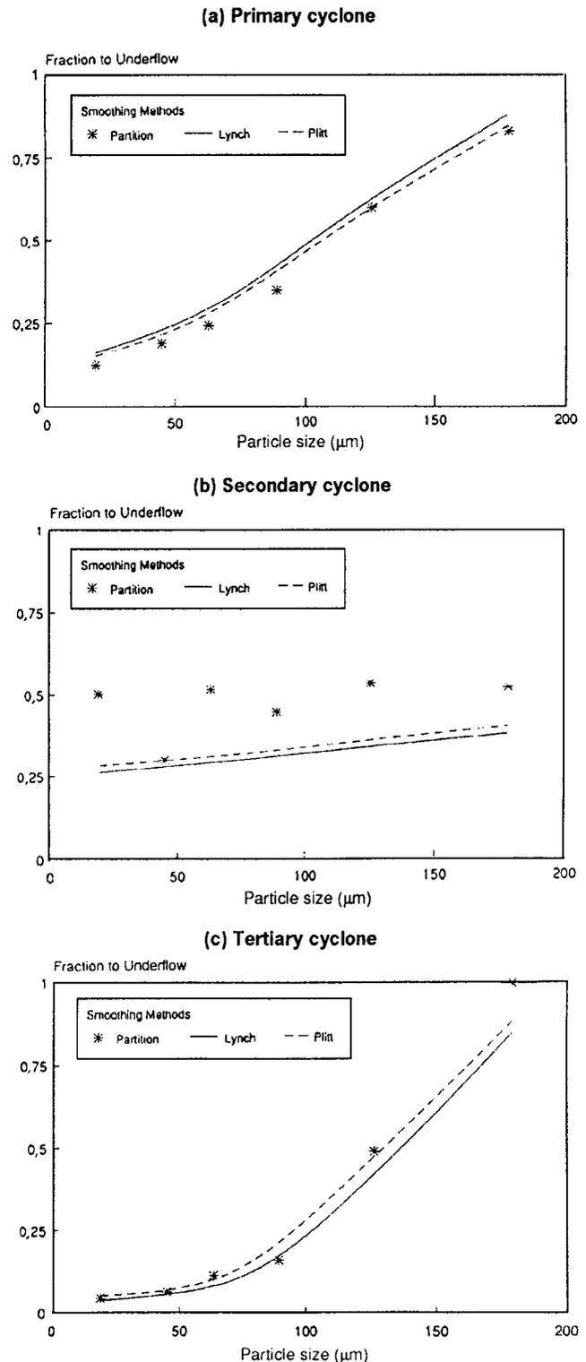
Figure 4—Partition curves obtained by different smoothing methods
