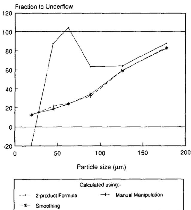
Figure 3—Partition curves obtained from plant data for a primary cyclone (Table I)
