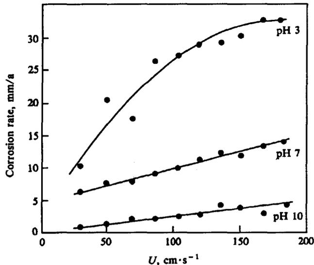
Figure 4—Influence of flow velocity on corrosion rate at different pH values (measured with the RCE)
