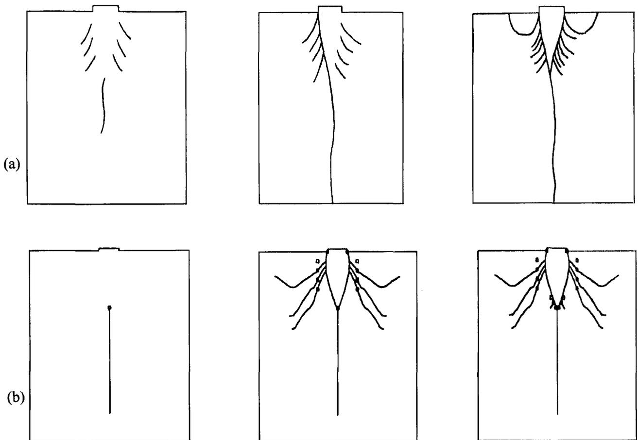
Figure 6—Fracture patterns under increased loading as observed in strip-punch tests: (a) physical modelling and (b) numerical modelling
