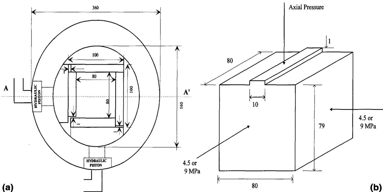
Figure 5—The poly-axial test frame (a) and a typical test specimen (b)
