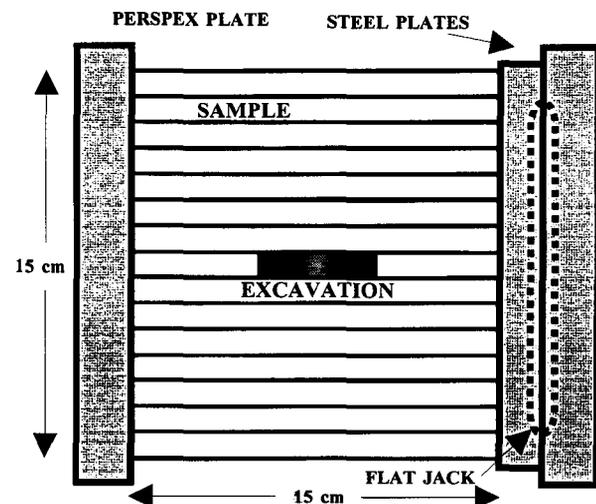
Figure 1—A schematic diagram of the plane-strain test rig
