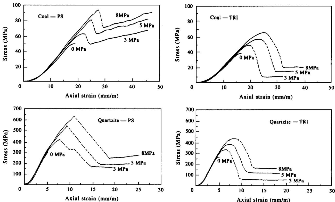
Figure 8—The differences in the stress–strain and strength characteristics of quartzite and coal tested under triaxial and plane-strain conditions
