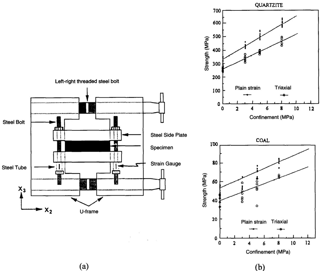
Figure 7—Plan view of the plane-strain test rig (a), and the strength characteristics obtained from axisymmetric and plane-strain testing (b)
