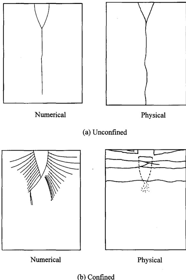
Figure 4—Fracture patterns obtained in the punch test
