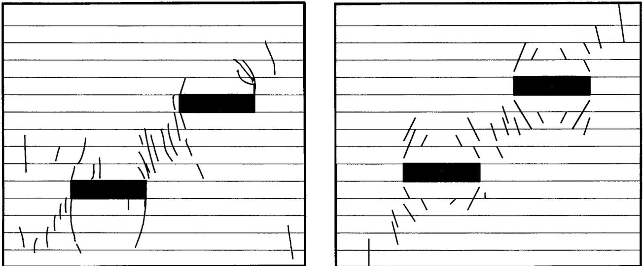
Figure 2—The fracture patterns obtained from plaster-of-Paris modelling (left) and numerical modelling (right)
