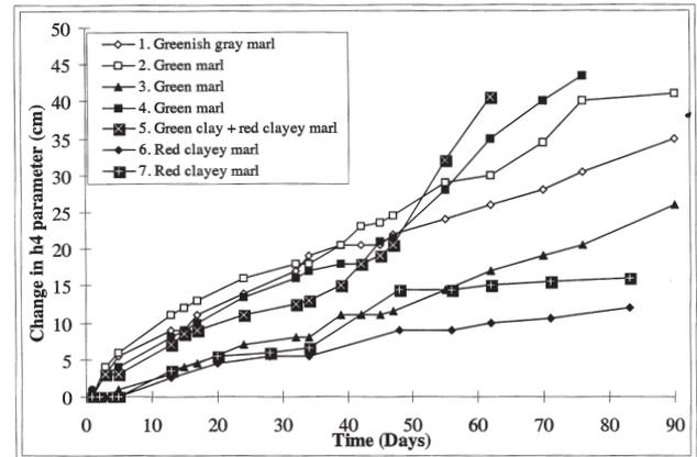
Figure 6—Change in  $h_4$  parameter as an indication of vertical closure in a period of three months
