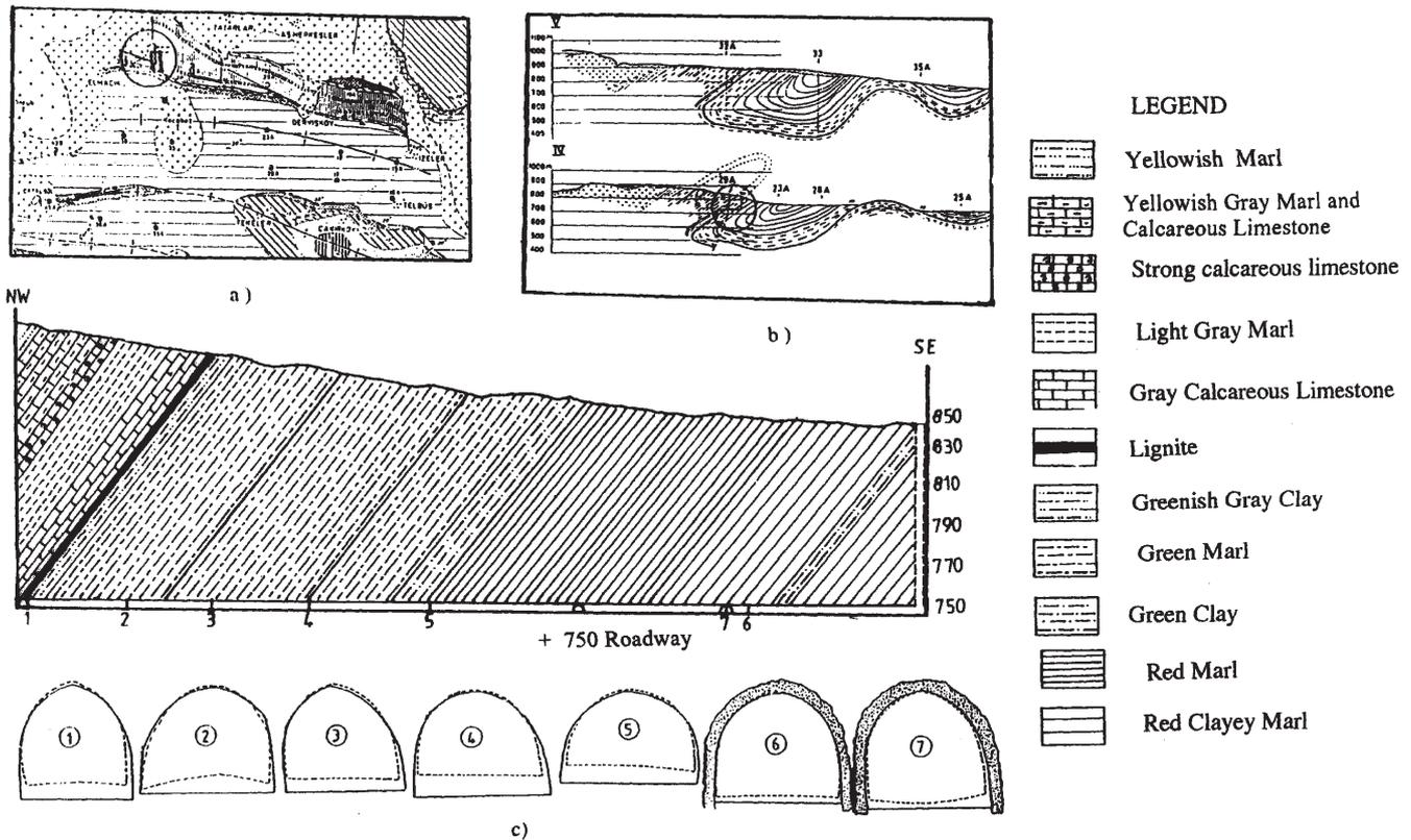
Figure 1—*a)* Geologic map of mine area, *b)* Cross-sectional view of mine area, *c)* Cross-sectional view of +750 roadway, locations of measurement stations and profiles of roadway after deformation
