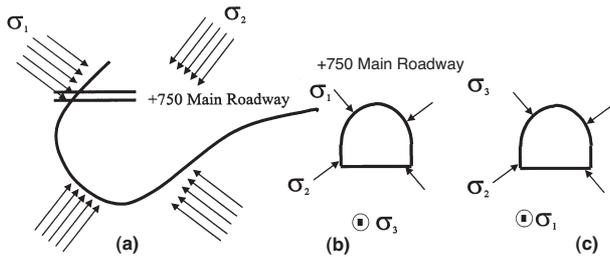
Figure 2—(a) Directions of principal stresses for the formation of existing asymmetric syncline and the position of +750 main roadway with respect to syncline, b) Directions of principal stresses affecting the roadway opened parallel to the syncline axis, c) Directions of principal stresses affecting the roadway opened normal to the syncline axis
