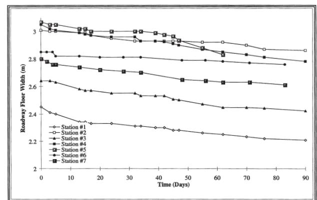
Figure 7—Change in the floor width at different convergence measurement stations in a period of three months
