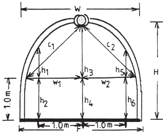
Figure 5—Method of convergence measurement
