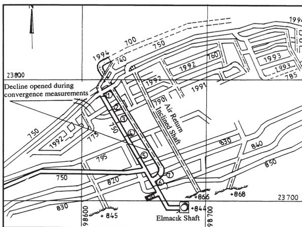
Figure 4—Locations of the convergence measurement stations on the mine plan
