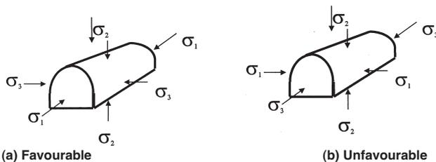
Figure 3—Relationship between roadway stability and the directions of principal stresses
