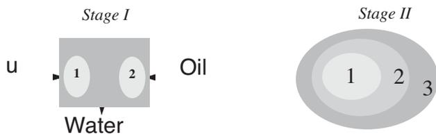
Figure 2—Stages I and II represent the state of the different components initially (I) and after contacting (II), where the coal-oil agglomerates are represented by oil in the diagram
