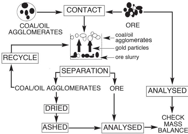
Figure 1—A Simplified flowdiagram of the Experimental Setup of the Coal Gold Agglomeration (CGA) process
