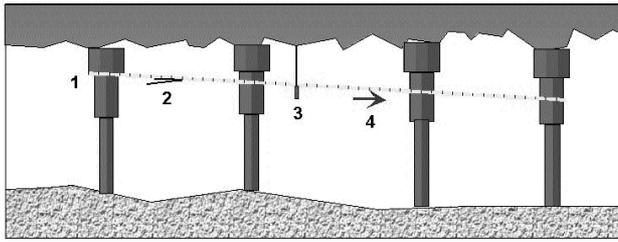
Figure 1—Sketch diagram showing method of data collection. (1) Tape is anchored tautly between two points, (2) Angle of tape and average dip of strata is recorded, (3) Distance between tape and hangingwall is measured (at each peak and trough for irregular profiles and at small regular intervals for periodic profiles), (4) Step 3 is repeated along the profile until the end-point is reached
