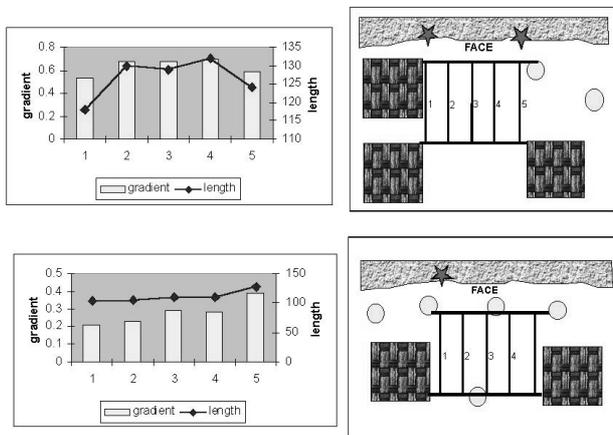
**Figure 5—Graphs on the left-hand side are the profile length and average gradients of the profiles measured around a preconditioned hole as shown by block diagrams on the right. The stars indicate the position of the preconditioning sockets from the previous day's blast. The profiles are 1 m long and 0.5 m apart. Note how both the average gradient and the profile length decrease towards the position of the socket, indicating a smoother hangingwall**
