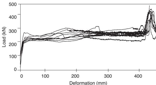
Figure 6—Force-deformation profiles of ten 1.2 m Rocprops; 15 mm/min deformation rate
