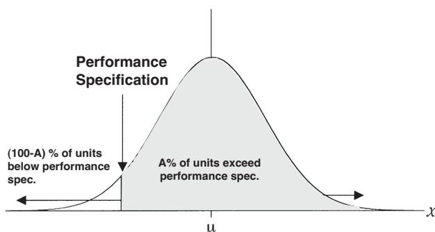
Figure 4—Probability density function sectioned according to performance specification
