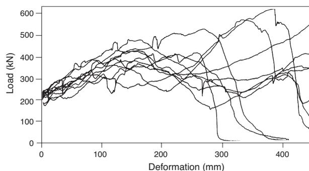
Figure 11—Force-deformation profiles of ten 1.6 m Loadmaster units; 15 mm/min deformation rate
