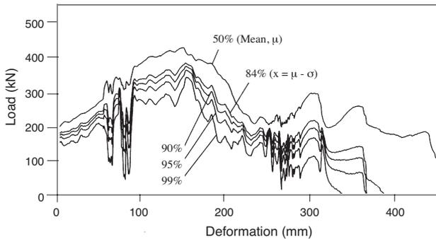
Figure 14—Loadmaster performance curves for various probabilities of exceeding the seismic support capacity ( $n = 1$ )
