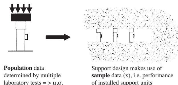
Figure 3—Schematic illustrating the difference between population and sample data
