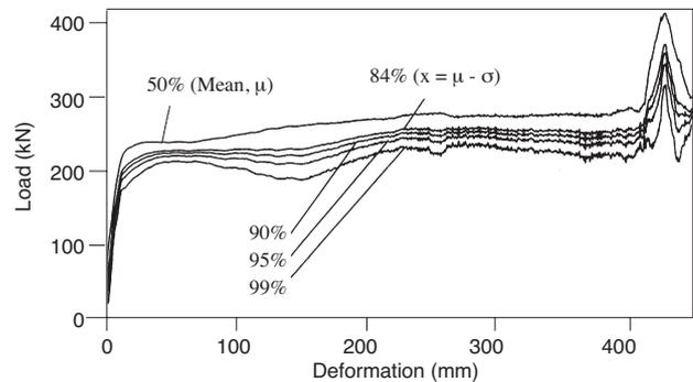
Figure 7—Rocprop performance curves for various probabilities of exceeding the support capacity ( $n = 1$ )
