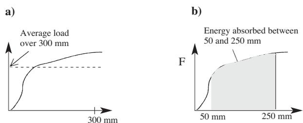
Figure 15a—Average load carrying capability up to a deformation of 300 mm, and (b) energy absorption between 50 mm and 250 mm deformation
