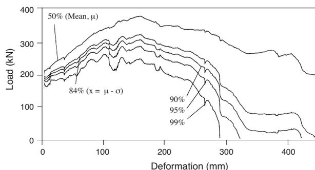
Figure 12—Loadmaster performance curves for various probabilities of exceeding the support capacity ( $n = 1$ )
