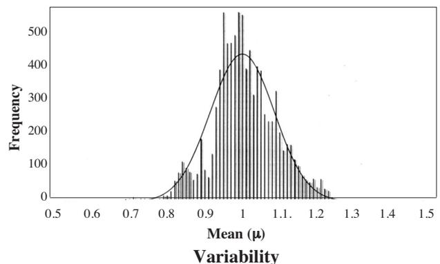
Figure 2—Histogram of the variability of support performance of a Rocprop elongate versus the normal probability distribution
