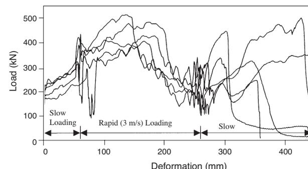
Figure 13—Force-deformation profiles of five 1.6 m Loadmaster units; 3 m/s deformation rate
