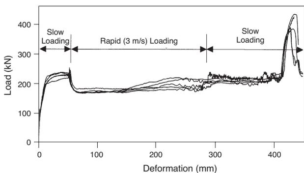
Figure 9—Force-deformation curves of five 1.2 m Rocprop; 3 m/s deformation rate
