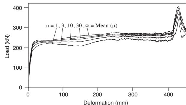
Figure 8—Performance curves for a support system comprising  $n = 1, 3, 10, 30$  and  $\infty$  Rocprop support units (95 per cent probability of exceeding performance curve)
