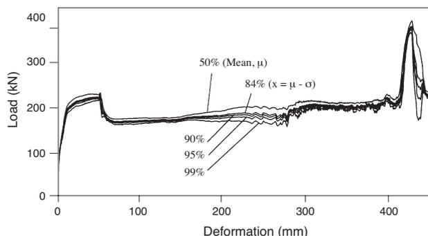
Figure 10—Rocprop performance curves for various probabilities of exceeding the seismic support capacity ( $n = 1$ )
