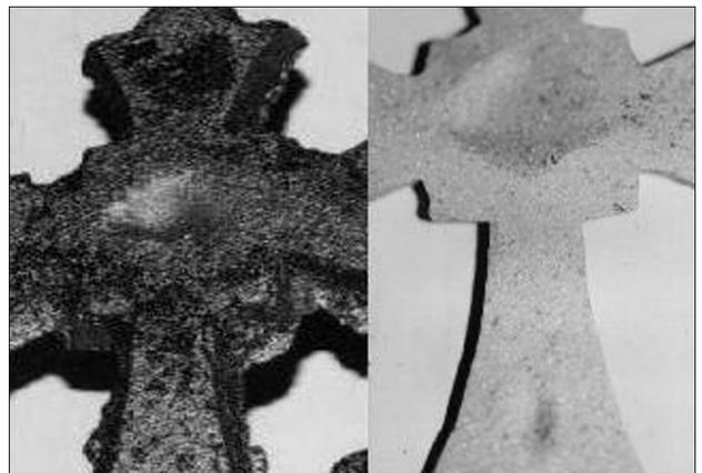
Figure 4—Two artifacts with Zinc composition greater than 40% showing shrinkage cavities (one in the as cast condition and the other after sand blasting)
