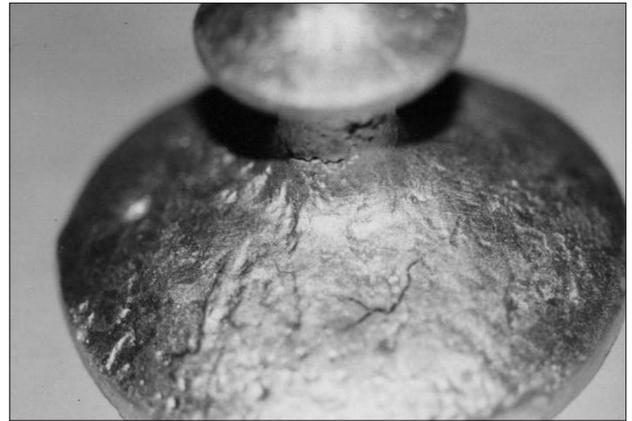
Figure 2—26% viscous Zinc casting showing cracks and cavities
