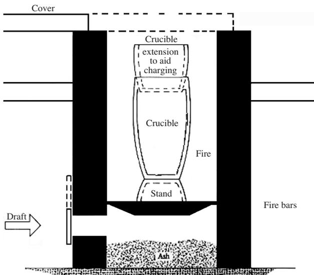
Figure 1—Typical coke-fired furnace
