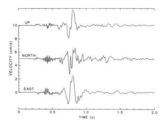
Figure 3—Ground velocity recorded at a surface site approximately 2.7 km from a mining-induced earthquake of *M*4.4 (from McGarr<sup>5</sup>)
