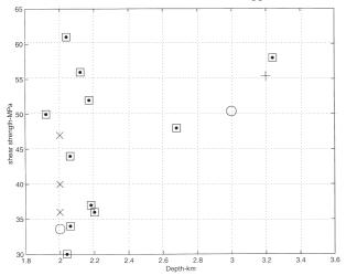
Figure 2—Large-scale shear strength of the Witwatersrand strata as a function of depth. The circles are estimates from [9]; the plus sign is an estimate based on results from McGarr *et al.*<sup>17</sup> and [8]; the x's are estimates from [10], involving the analysis of fault gouge; finally, the squares are estimates (Table I) derived from moment tensors of mining-induced earthquakes
