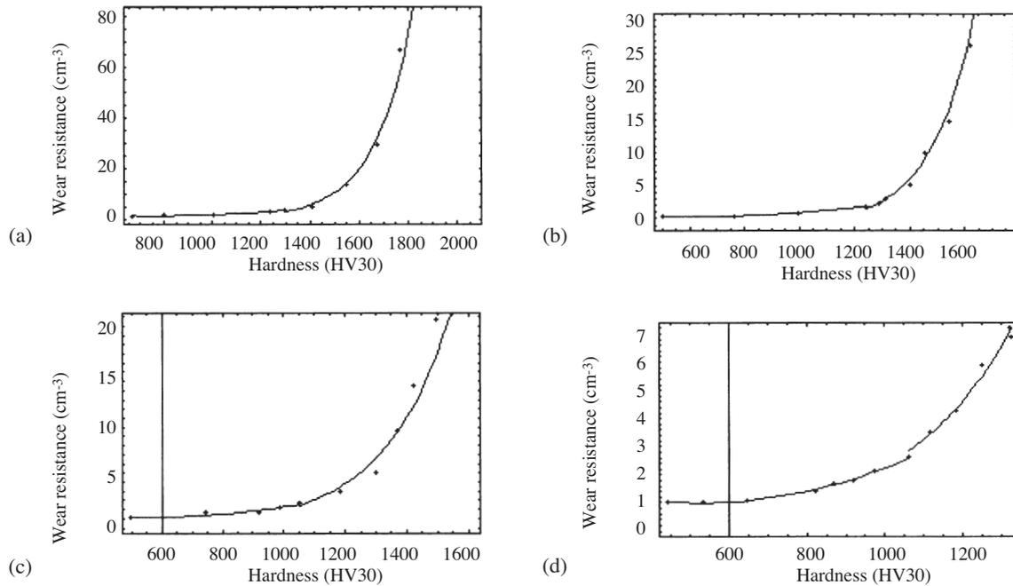
Figure 2—Plots of the abrasion resistance versus the hardness of the four groups of WC-Co grades listed in Table I (a) group UF; (b) group F; (c) group M; (d) group C. The points are the experimental data and the continuous curve sections are the curve sections that best fit the data as determined by a least squares fit. The analytical expressions of the various curve sections are given in Table III
