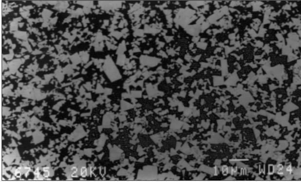
Figure 1—Typical microstructure of a WC-Co alloy: the white phase consists of WC grains of 3  $\mu\text{m}$  mean size and the black phase is the cobalt binder (by courtesy of Mr Thabo Sebeya)
