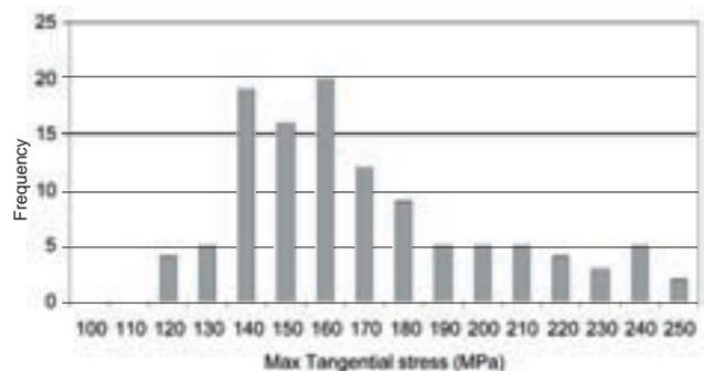
Figure 7—Distribution of the maximum tangential stress acting on the rockpass
