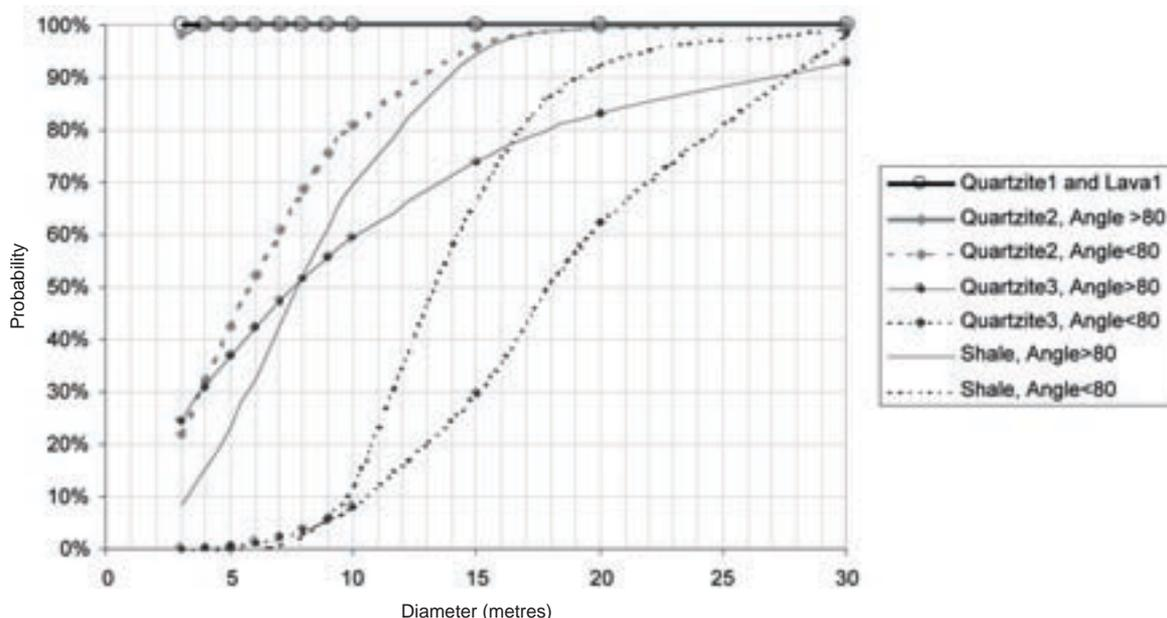
Figure 14—Probability of a rockpass not exceeding a given diameter for various rock types and favourable versus unfavourable orientations
