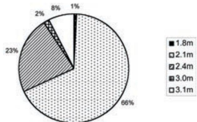
Figure 4—Excavated pass diameters
