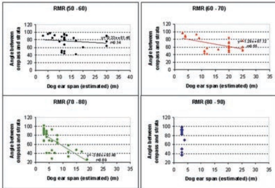
Figure 16—Relationships between pass orientation relative to strata dip and dog ear spans
