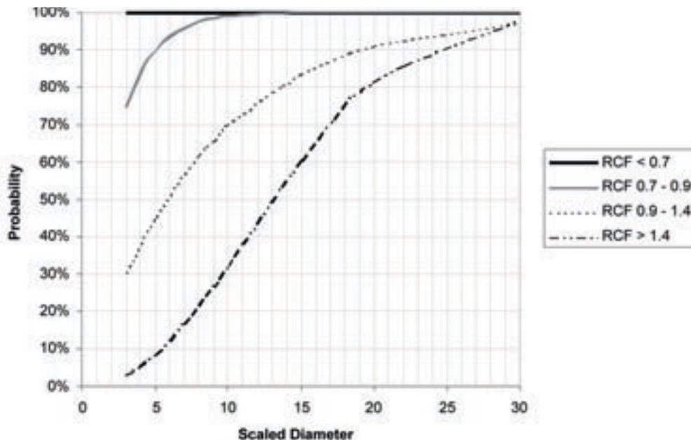
Figure 15—Probability of a rockpass not exceeding a given diameter for ranges of rockwall condition factor (RCF)
