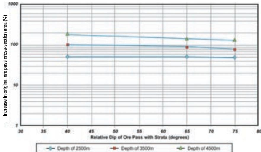
Figure 5—Influence of pass orientation relative to strata orientation on pass stability at various depths for a 1.8 m diameter pass (with dog-earing)
