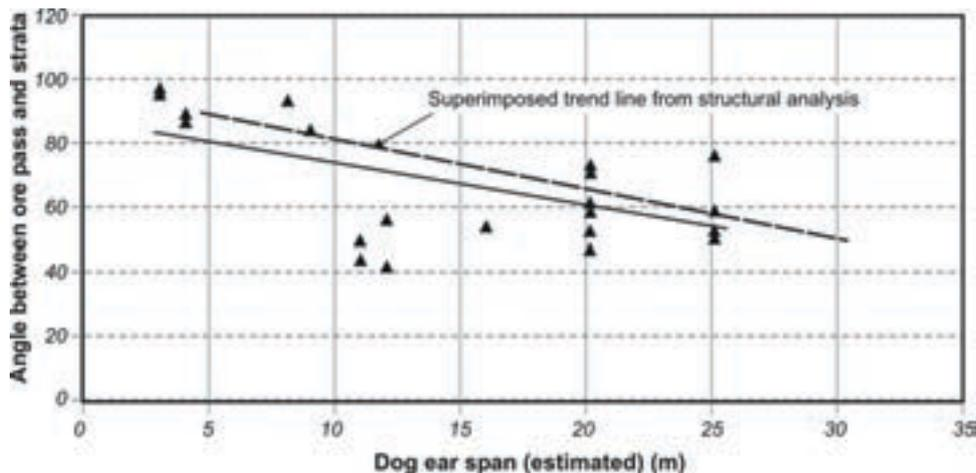
Figure 7—Estimated dog ear spans vs. angle between pass and strata (RMR 60–70)
