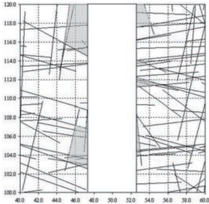
Figure 2—Generated joint traces in a vertical section through a rockpass
