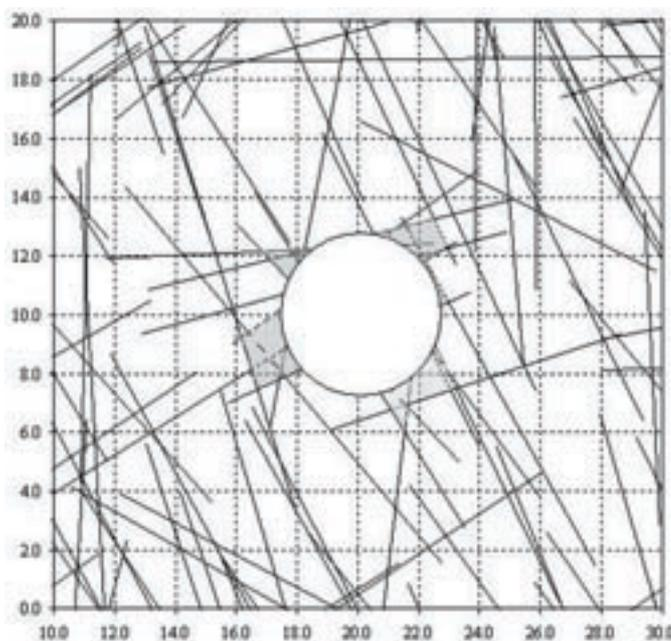
Figure 1—Generated joint traces in a horizontal section through a rockpass
