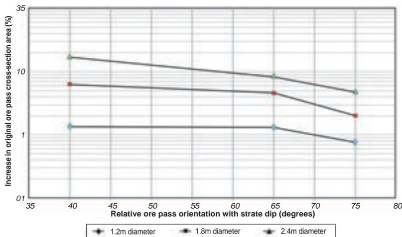
Figure 4—Influence of pass orientation relative to strata orientation with different diameters (no dog-earing)
