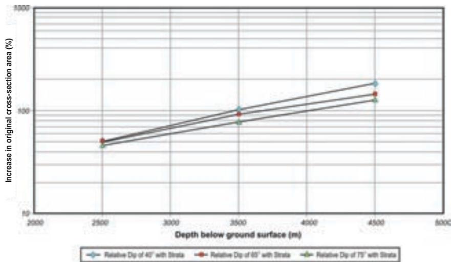
Figure 6—Influence of pass depth for a 1.8 m diameter pass (with dog-earing)
