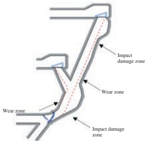
Figure 8—Damage zones in an ore pass
