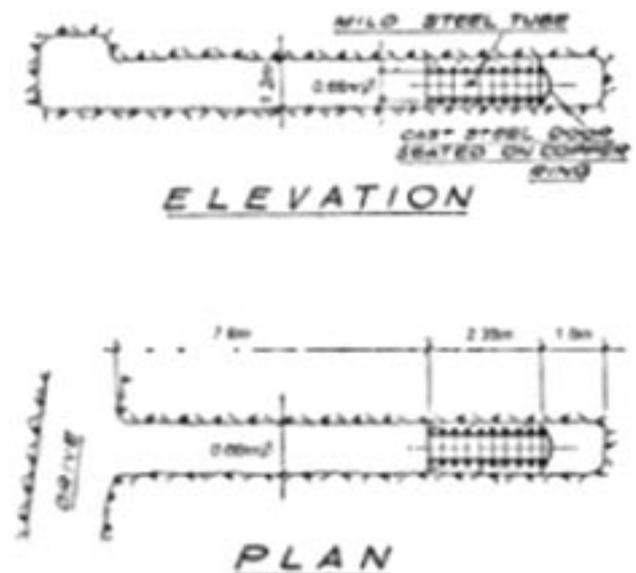
Figure 4—Experimental plug, West Driefontein
