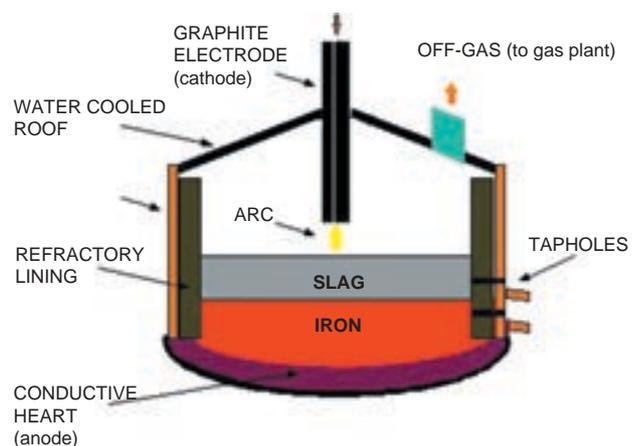
Figure 3—Schematic of DC-arc furnace
