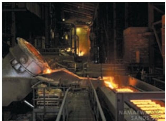
Figure 8—Pig casting
