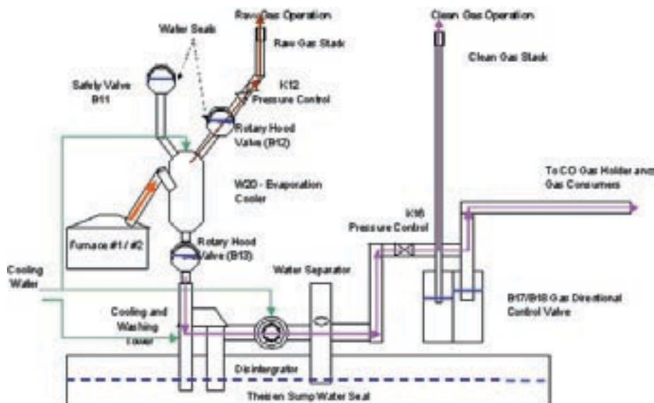
Figure 4—Gas cleaning plant
