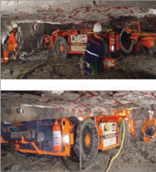
SMC MKII drill rig and roofbolter at Waterval
