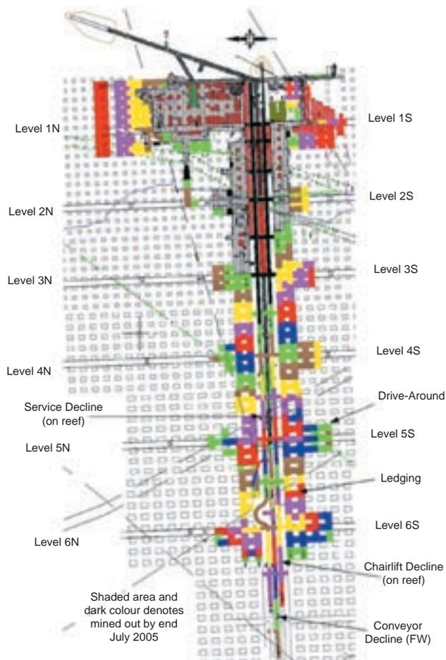
Figure 5—The TRP bord and pillar layout for mechanized mining with the level down dip and strike roadways
