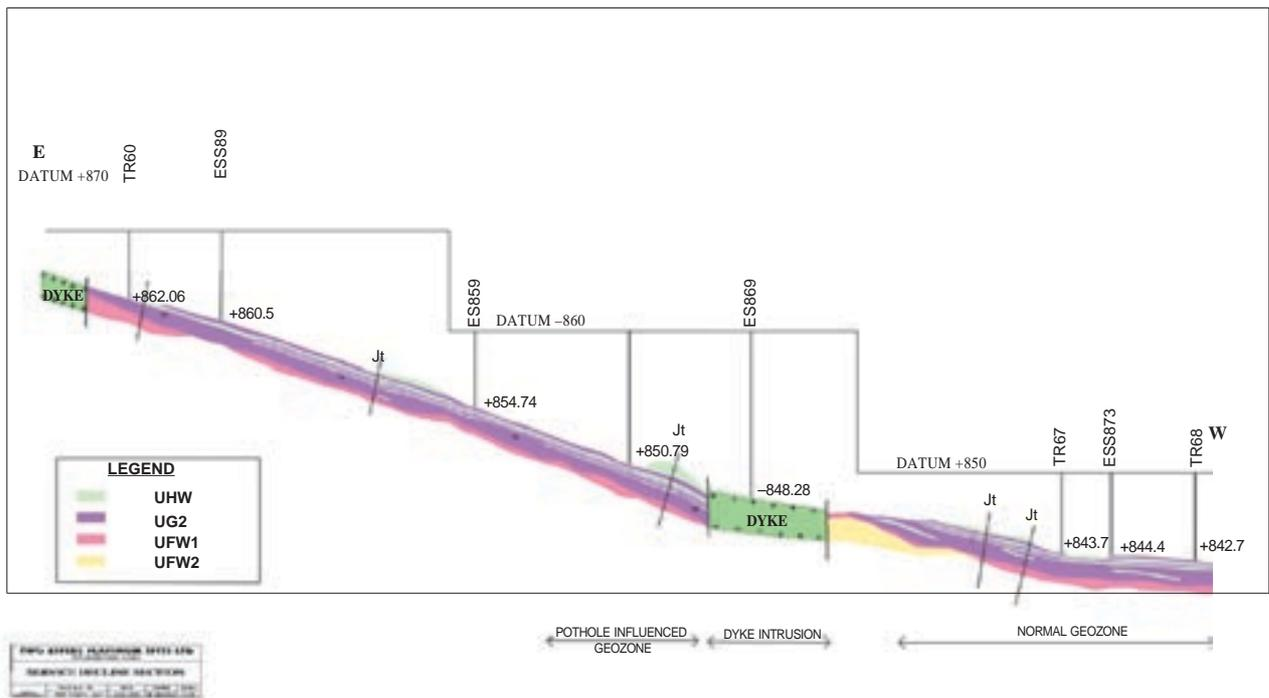
Figure 4—A dip section along part of the on reef service decline, showing the morphology of the reef. Note sections of hangingwall over break where the dip is slightly steeper than average
