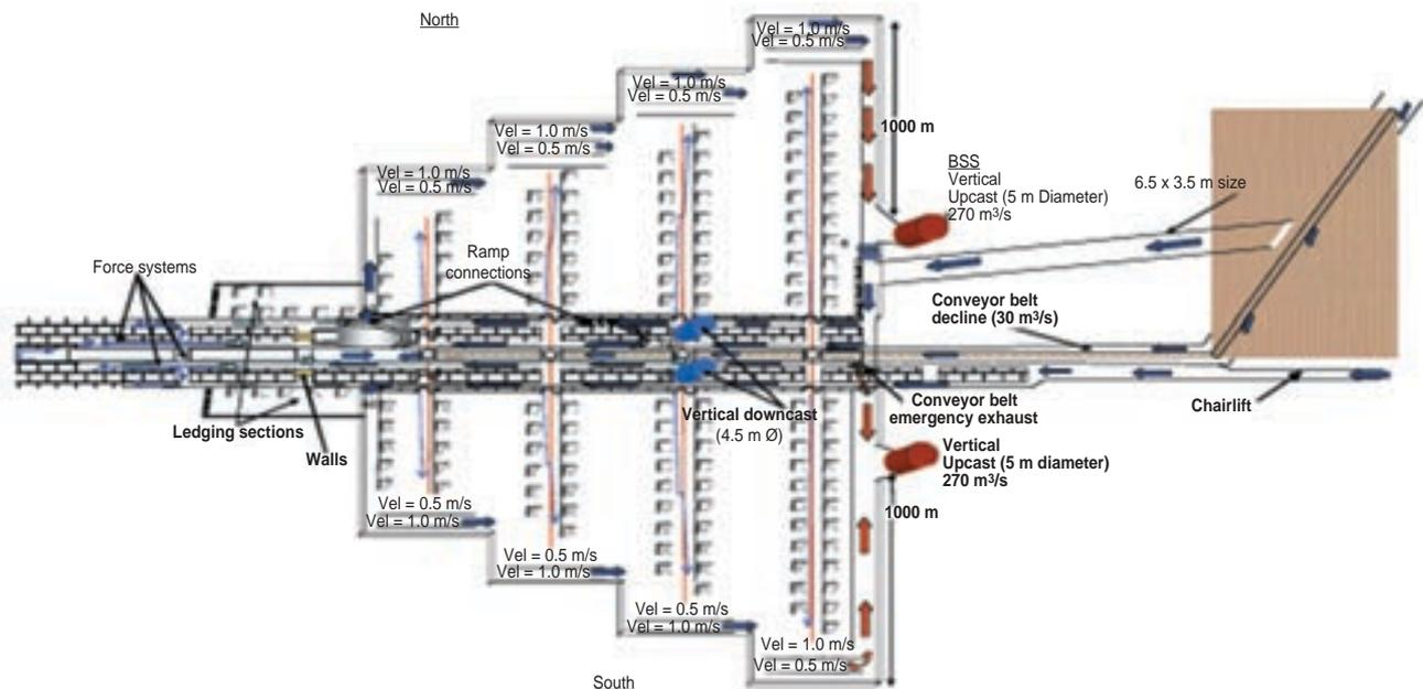
Figure 9—The steady state ventilation design and layout at TRP
