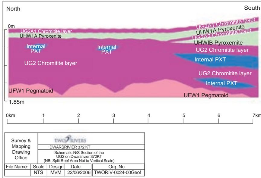
Figure 3—A section N-S of TRP showing the UG2 layer, leaders and pyroxenite partings to the south (after R. Hornsey, unpublished 2003)
