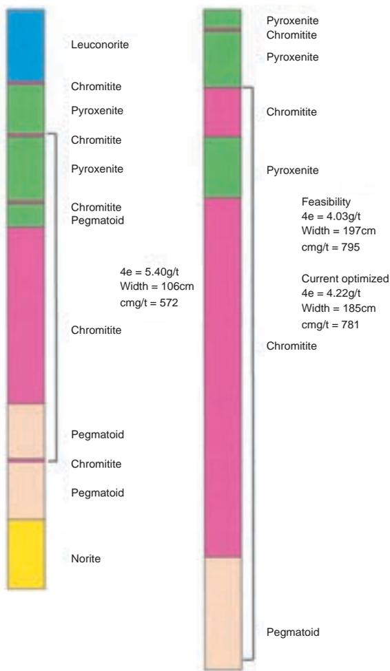
Figure 2—A stratigraphic comparison between the Modikwa Mine cut (left), and TRP mine cut (right). The Modikwa cut is equivalent to the lower UG2 split reef facies in the southern portion of the Two Rivers farm (see Figure 3)
