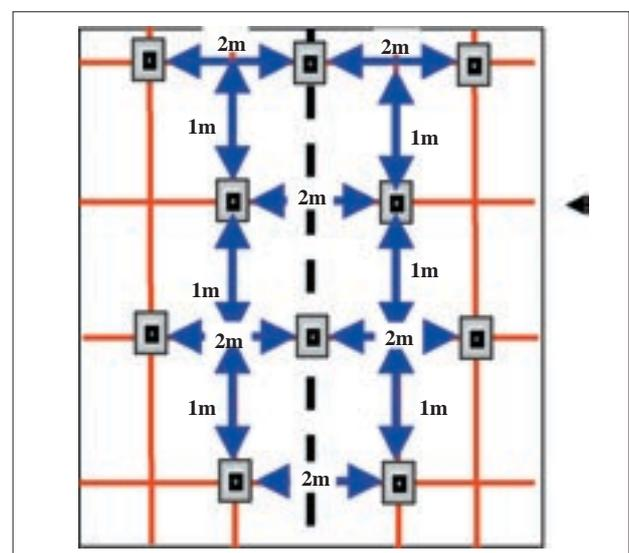
Figure 8—Stope support pattern at Two Rivers Platinum
