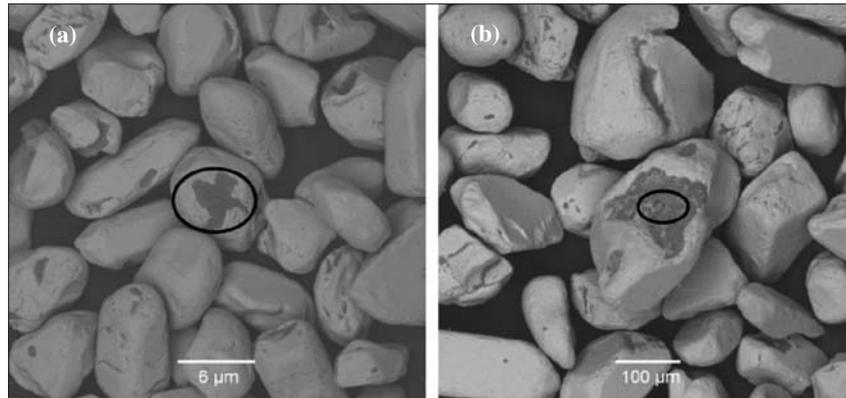
Figure 2—Back-scattered electron images showing typical coatings (circled in black) existing on the more conductive (a) and non-conductive (b) zircon particles (Magnification: Figure 2(a) x180 at 15 kV acceleration voltage; Figure 2(b) x150 at 15 kV acceleration voltage)
