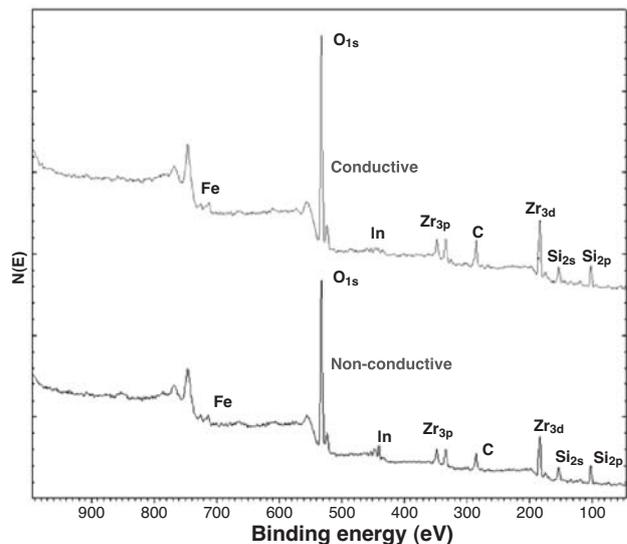
Figure 1—XPS surveys obtained during the XPS analysis of the zircon particles from the different streams
