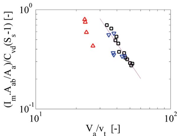
Figure 4—Stratification ratio ( $\mu$  - 0.37 mm sand in the 150 mm pipe,  $\tilde{N}$  - 0.3 mm sand in the 105 mm pipe,  $\Delta$  - 0.56 mm sand in the 105 mm sand, line-correlation, Equation [4], for  $K = 730$  and  $n = 2$ )
