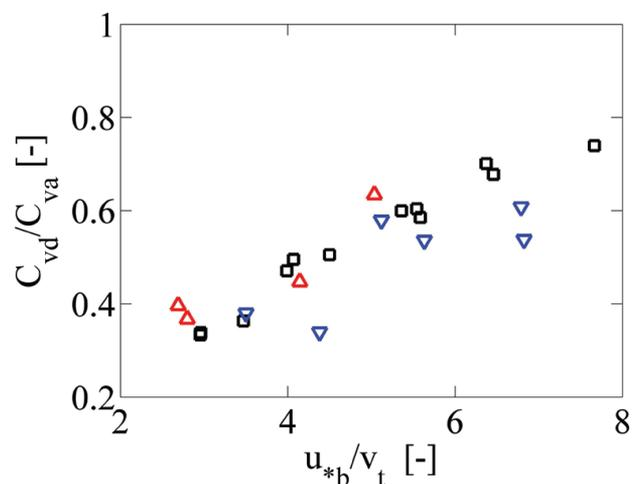
Figure 2—Slip ratio in flow above stationary bed (squares—0.37-mm sand in the 150-mm pipe, downward-pointing triangle—0.3-mm sand in the 105-mm pipe, upward-pointing triangle—0.56-mm sand in the 105-mm sand)
