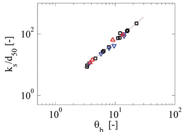
Figure 5—Relative hydraulic roughness of the top of the stationary bed (squares—0.37-mm sand in the 150-mm pipe, downward-pointing triangle—0.3-mm sand in the 105-mm pipe, upward-pointing triangle—0.56-mm sand in the 105-mm sand)
