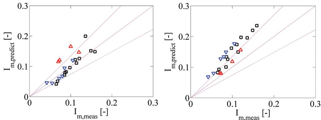
Figure 6—Comparison of measured and predicted  $I_m$  (left—here presented model, right—Pugh-Wilson model, dashed line—35% deviation from the  $I_{m,predict} = I_{m,meas}$ )
