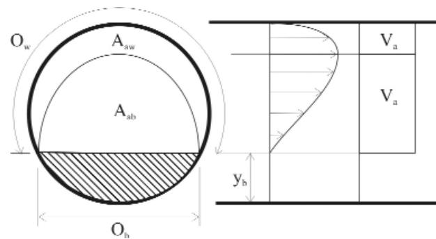
Figure 1—Schematic geometry of pipe cross-section and schematic distribution of velocity in flow of slurry through discharge area above stationary bed
