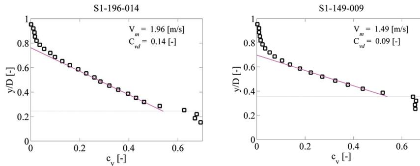
Figure 3a—Concentration profiles in the 150-mm pipe (squares—measured local concentrations, lines—best-fit lines)
