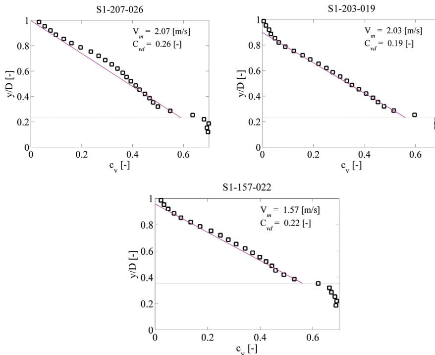
Figure 3b—Concentration profiles in the 150-mm pipe (squares—measured local concentrations, lines—best-fit lines)
