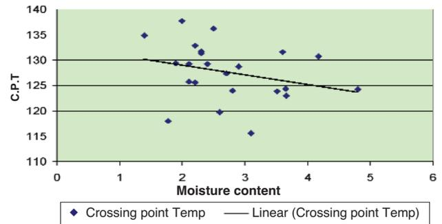
Figure 12—Inherent moisture content versus Crossing Point Temperature
