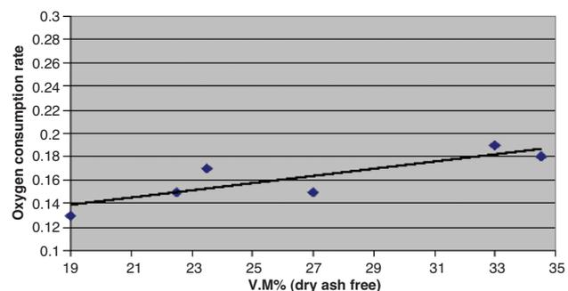
Figure 1—Rate of oxidation and rank of coal
