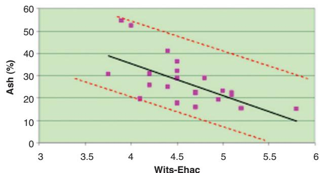
Figure 15—The effect of Ash % on the Wits-Ehac index
