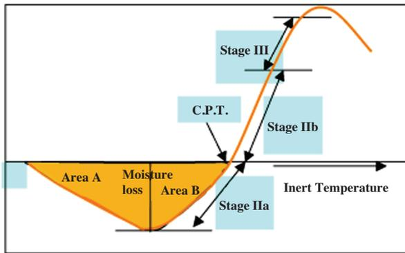
Figure 7—DTA thermogram showing important regions used in calculations
