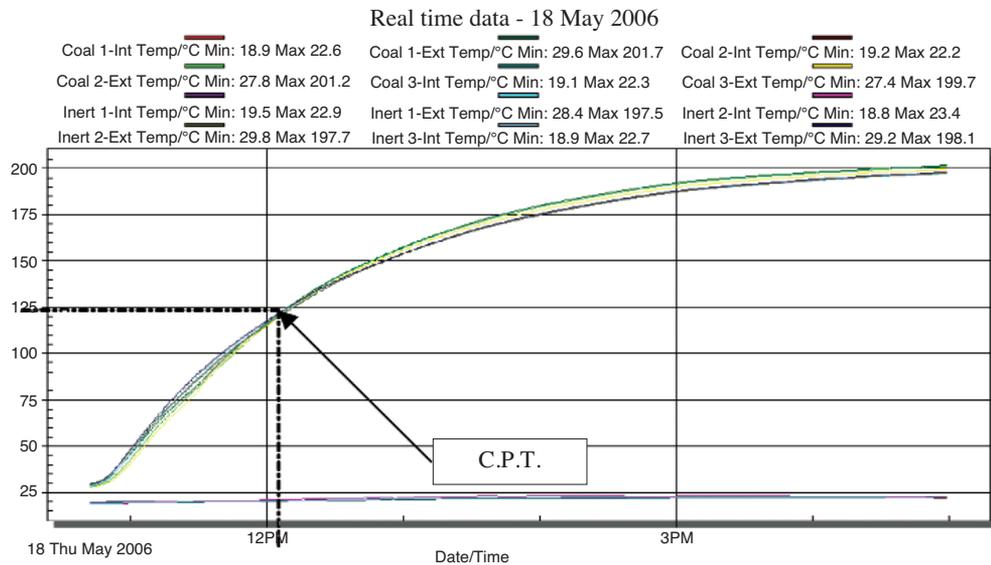
Figure 3—Temperature curves of coal and inert material showing crossing point temperature
