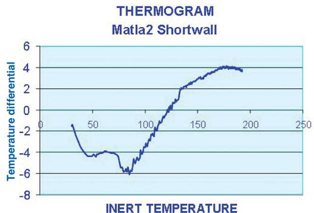
Figure 4—A typical D.T.A. thermogram obtained for a coal sample
