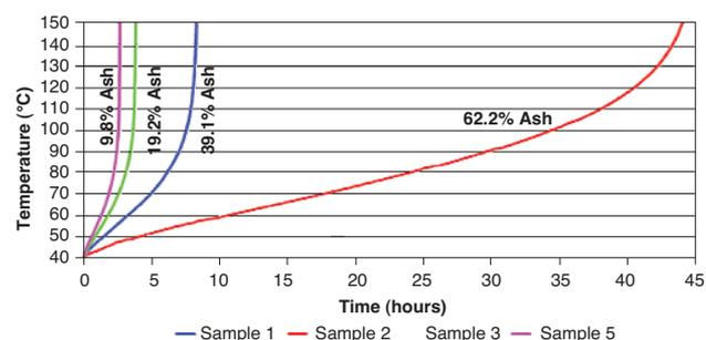
Figure 2—The effect of ash content on time to self-heating of coal (Blazak, 2001)
