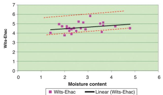
Figure 13—Inherent moisture content versus Wits-Ehac Index
