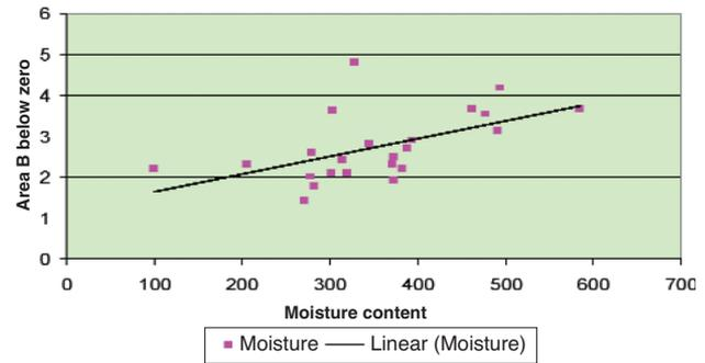
Figure 10—The total area under zero differential is compared with inherent moisture content
