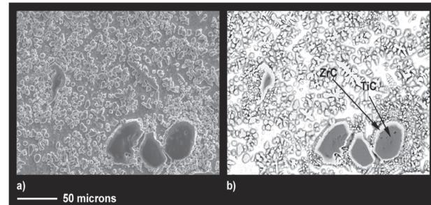
Figure 10—SEM Micrograph showing the decomposition of TiC particles
