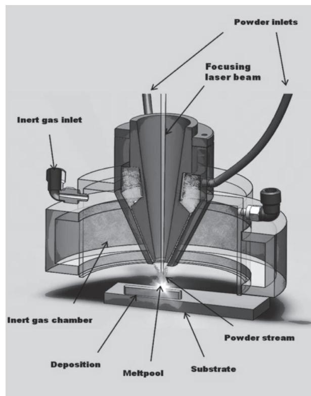
Figure 2—Schematic diagram of coaxial deposition nozzle (CSIR)
