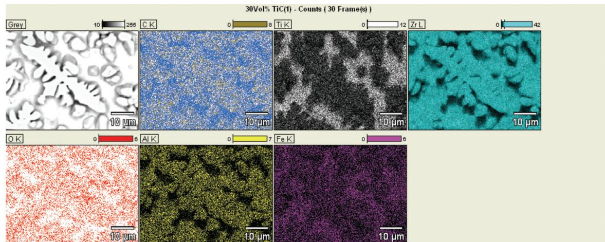
Figure 11—EDS element map of dendritic ZrC and dentritic TiC matrix
