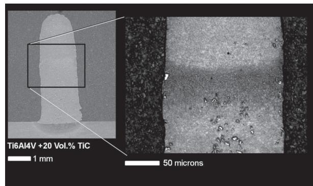
Figure 4—Optical macro- and micrographs showing microstructure transition occurring in laser-deposited MMCs
