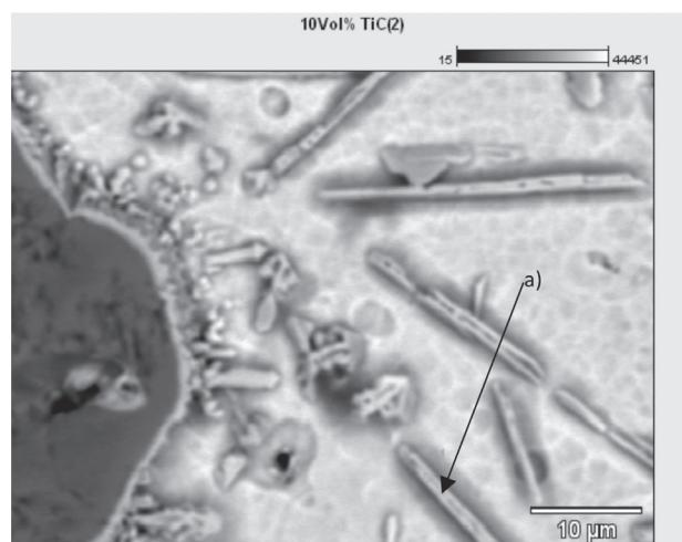
Figure 12—Backscattered SEM micrograph showing decomposition of TiC
