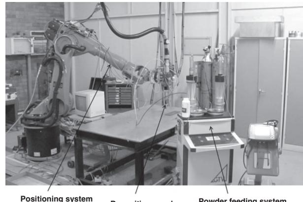
Figure 1—Photograph of the laser metal deposition facility
