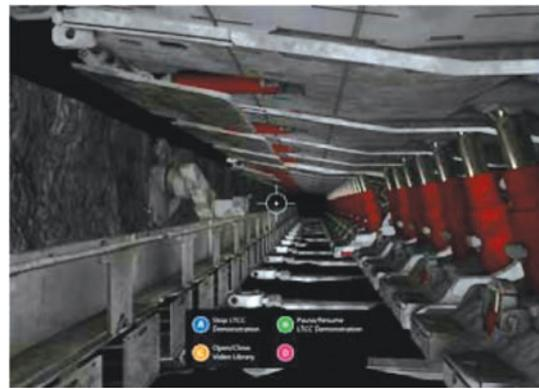
Figure 7—Screenshot from the Longwall Top Coal Caving module
