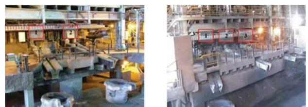
Figure 7—Two and three tap-hole layouts
