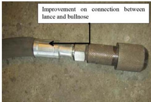
Figure 16—New bullnose design for oxygen pipe
