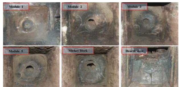
Figure 14—Cold face of tapping modules
