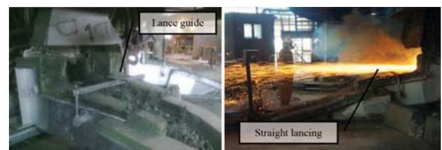
Figure 12—V-shaped lance guide ensuring straight lancing
