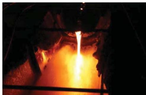
Figure 4 – Slag granulation
