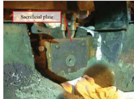
Figure 17—Sacrificial plate on copper faceplate
