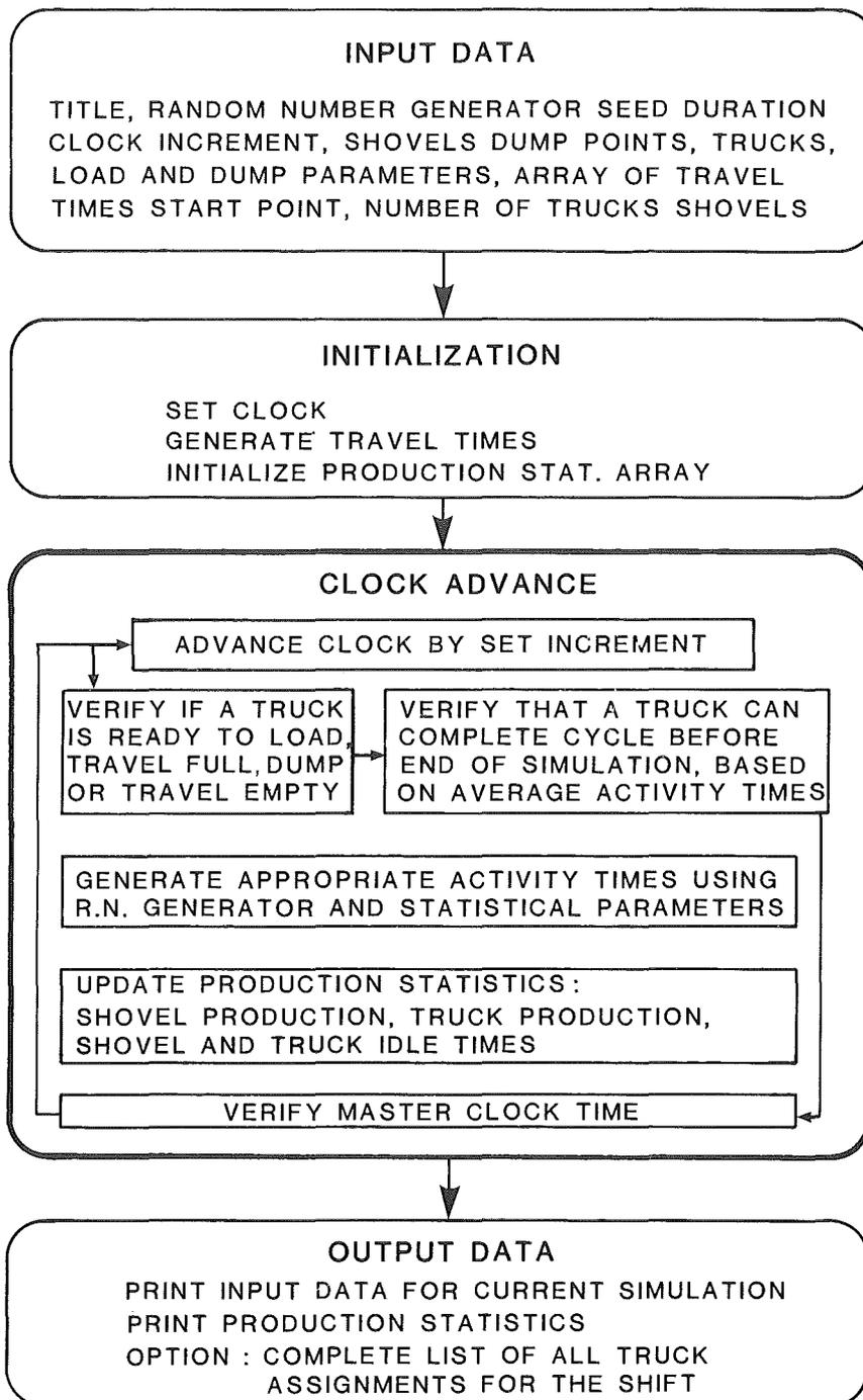
FIGURE 2. General structure of simulation program
