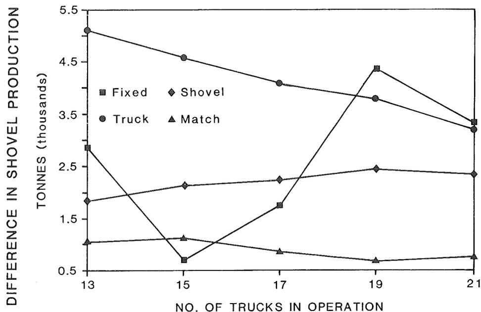
FIGURE 7. Maximum difference in shovel production<sup>6</sup>
