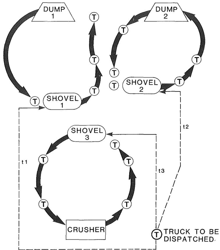
FIGURE 3. Maximize truck dispatching rule
