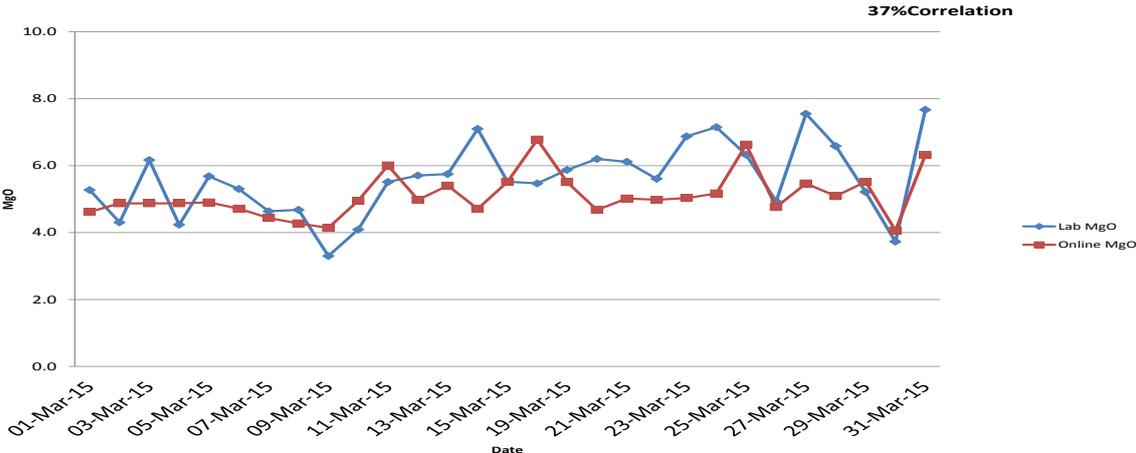
Figure 11. Comparison of MgO analyses from the laboratory and from the on-line analyzer.
