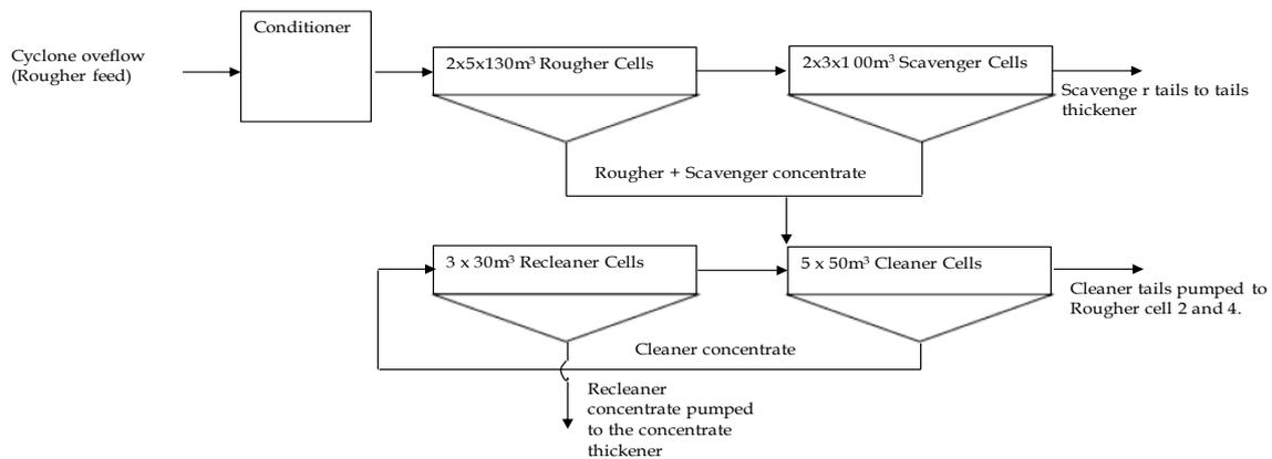
Figure 1. The MMZ plant flotation circuit overview.
