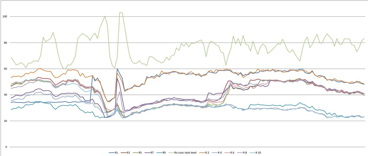
Figure 6. Rougher cells air flow rate tracking vs rougher concentrate level.
