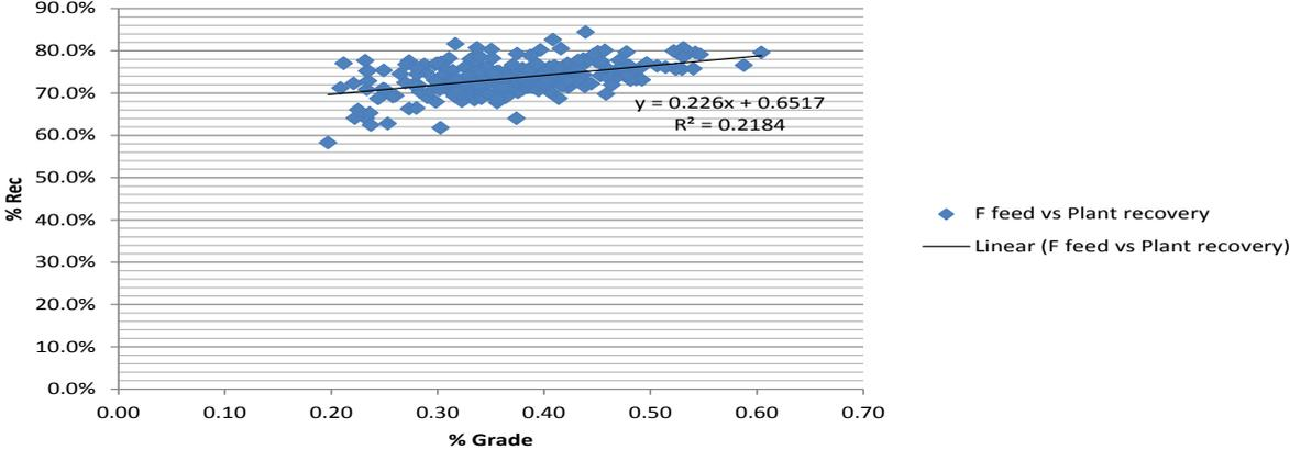
Figure 9. Plant recovery vs. head grade.
