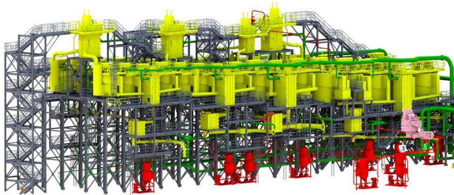
*Figure 2. Example of current molybdenum flotation plant.*
