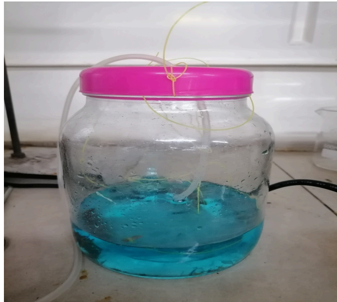
Figure 6. Copper leach solution obtained in stage 1 leaching of metallic sheets using 0.4\text{M}\text{CuSO}_4+4\text{M}\text{NaCl}+0.5\text{M}\text{H}_2\text{SO}_4 solution, room temperature and stirring speed of 500 rpm.
