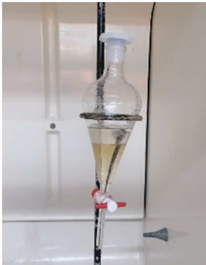
Figure 8. Solvent extraction of gold using 2 ethyl-hexanol in toluene before stripping in 1.0 M NaOH.
