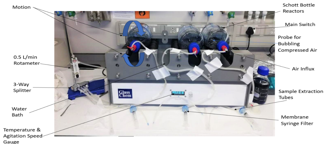
Figure 5. Three parallel Schott bottle reactors, with identical leaching conditions, that were used in the leaching reaction involving the bottle roller.
