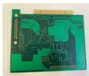
Figure 3. Custom-made PCB top surface layer (Layer 1). Figure 4. Custom-made PCB bottom surface layer (Layer 4).
