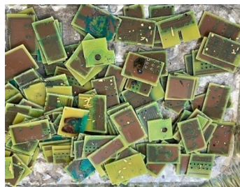
Figure 15. Untreated PCBs in experiment 6 after leaching with waste etchant.
