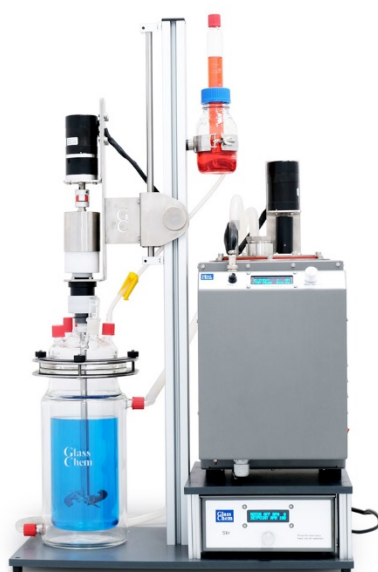
Figure 2. The GlassChem reactor configuration for zinc leaching from sphalerite concentrates using ammonia.
