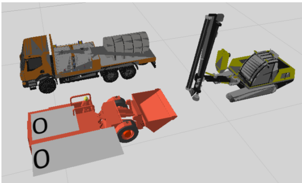
Figure 5. Moveable objects indicating LHD in red, drill rig in yellow and charging rig in brown (Source: Oosthuizen, 2021).
