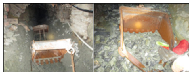
Figure 7—Double (left) and single (right) scraper configuration in cleaning in a strike gully (photos by author)
