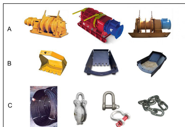
Figure 6—Various components of the scraper winch system including a winch, scraper, and winch rope (Bafotech, n.d.; Cape Gate, n.d.; Galison Manufacturing, n.d.; Powerflow Scraper Winches, n.d.; Toco Lifting, n.d.; Wolfram Mining Supplies, 2024)
