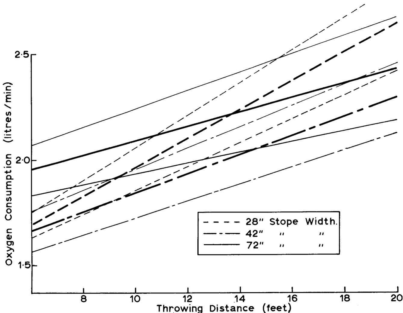
Fig. 3—Influence on oxygen consumption of distance of throw
