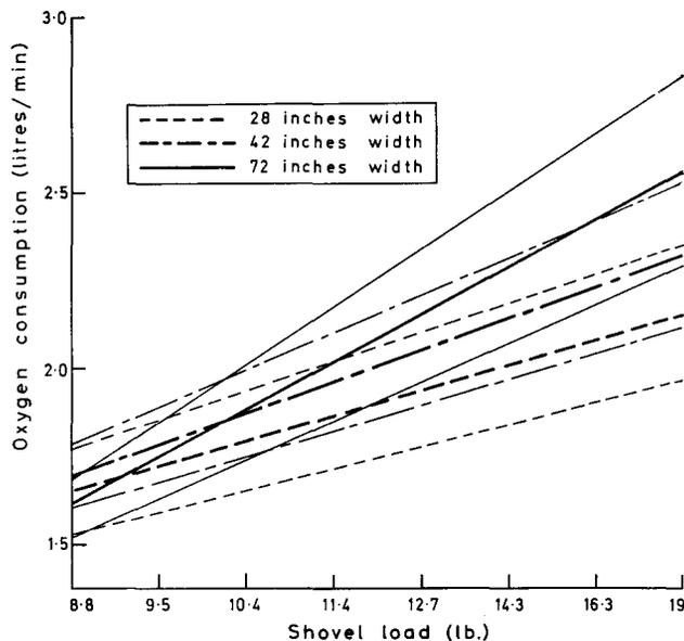
Fig. 4—Influence on oxygen consumption of shovel load
