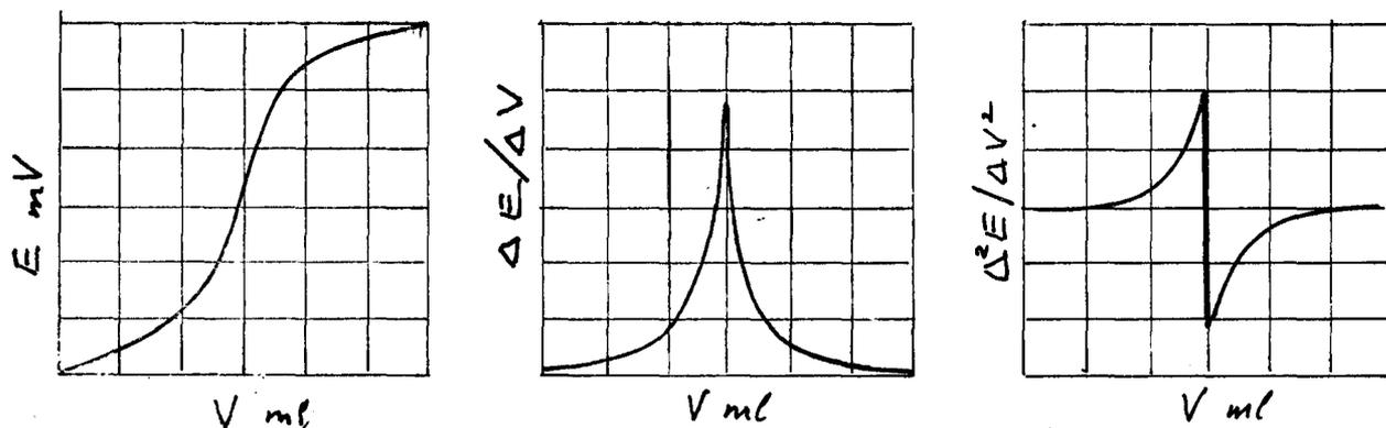
Fig. 1—Typical precipitation titration curves
