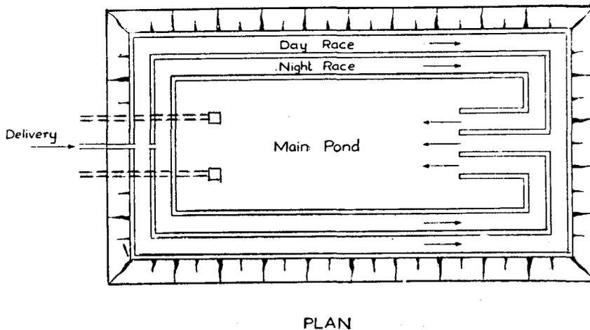
Fig. 2—Slimes-dam race system (from Adamson<sup>1</sup>)
