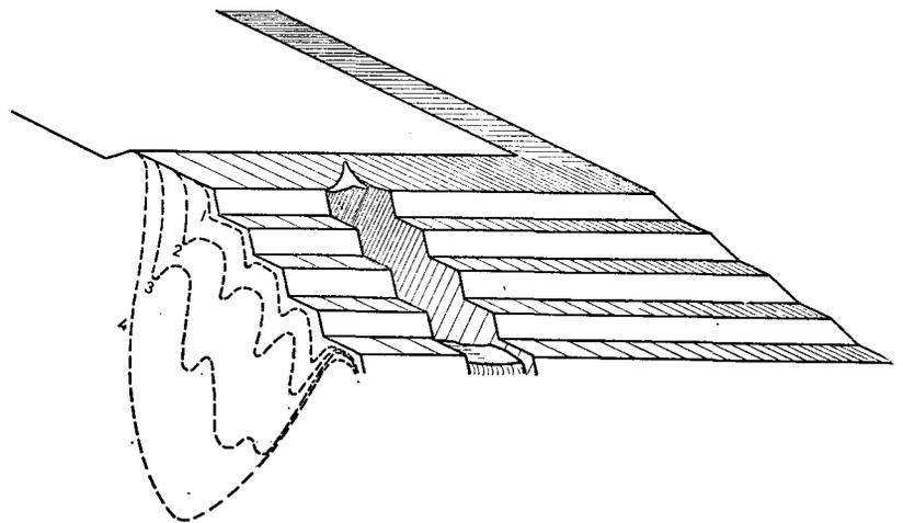
Fig. 7—Successive stages of erosion on a slimes-dam wall
