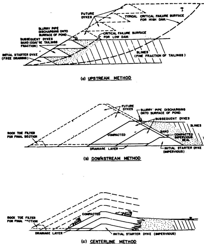
Fig. 6—Methods of tailing-dam construction (from Brawner and Campbell<sup>8</sup>)
