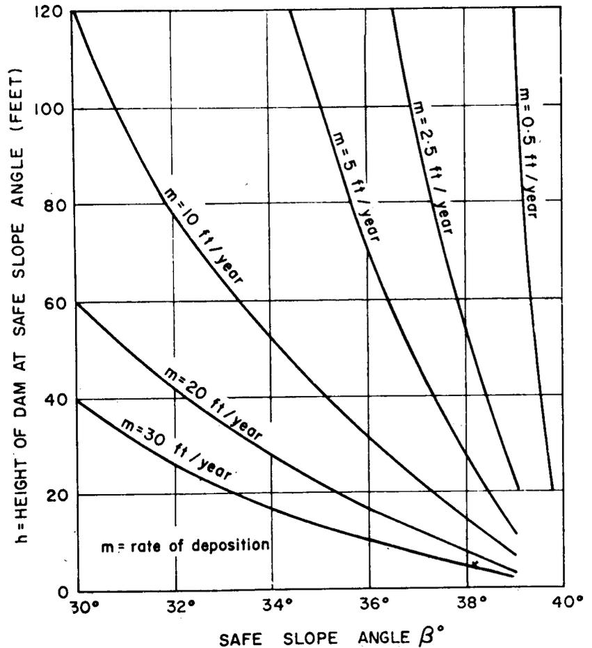
Fig. 4—Design graph for slimes dams having an impervious base (from Blight<sup>11</sup>)
