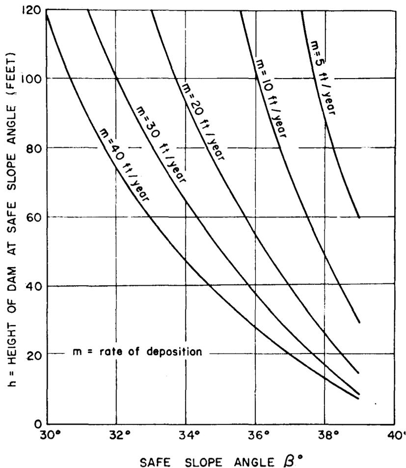
Fig. 5—Design graph for slimes dams having a pervious base (from Blight<sup>11</sup>)
