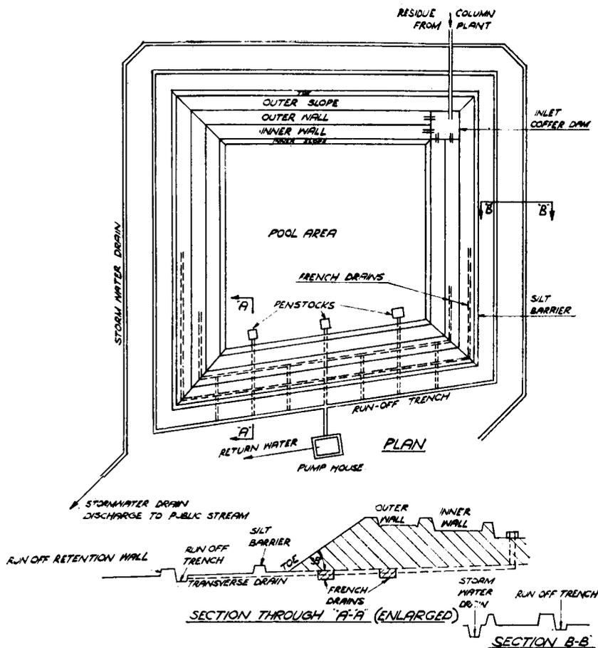
Fig. 3—Plan of a slimes dam and section of a wall (from Adamson<sup>1</sup>)
