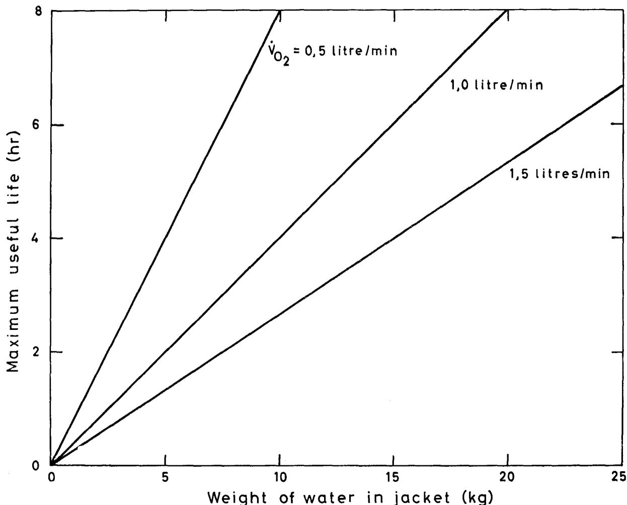
Fig. 3—Maximum useful life (in hours) assuming all metabolic heat is absorbed in the jacket and no heat is stored in the body
