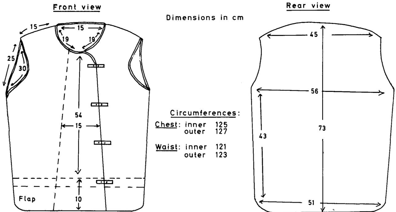
Fig. 2—Dimensions of outer jacket
