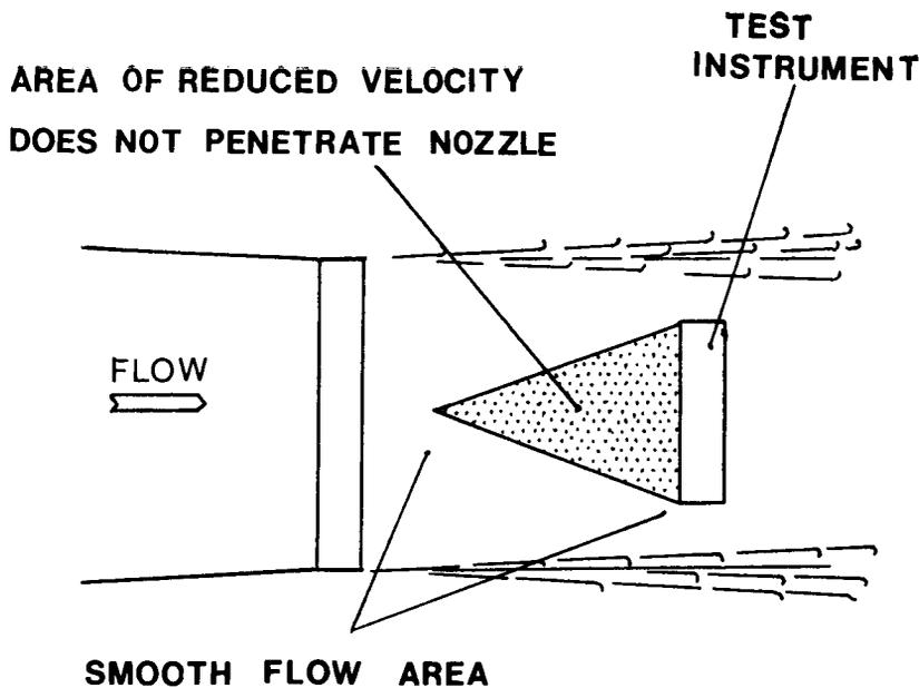
Fig. 2—Substantially parallel flow at outlet
