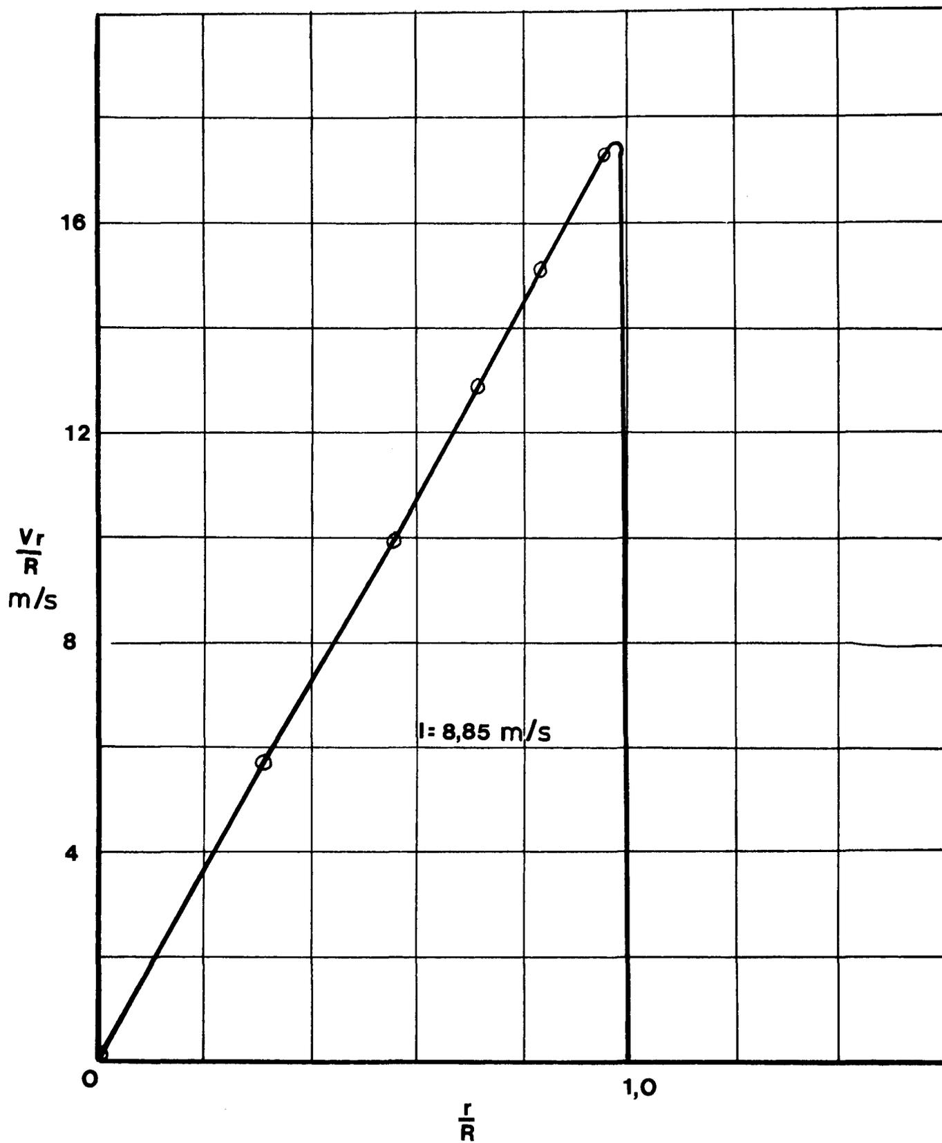
Fig. 4—Determination of I by planimeter integration
