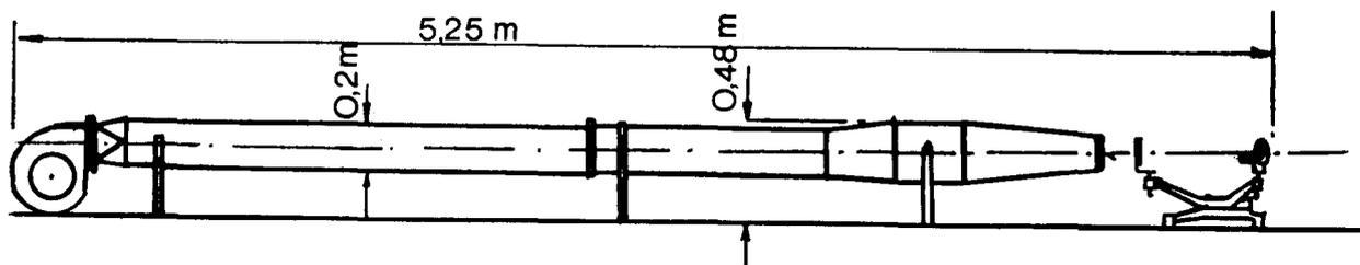
Fig. 1—Arrangement of wind-tunnel assembly
