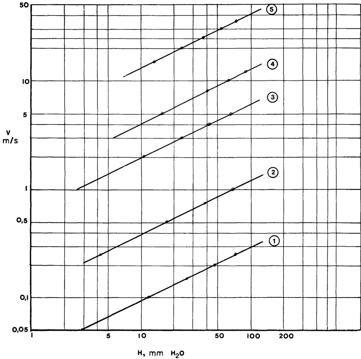
Fig. 6—Final calibration curves for five orifice plates (density 1,03 kg/m<sup>3</sup>)
