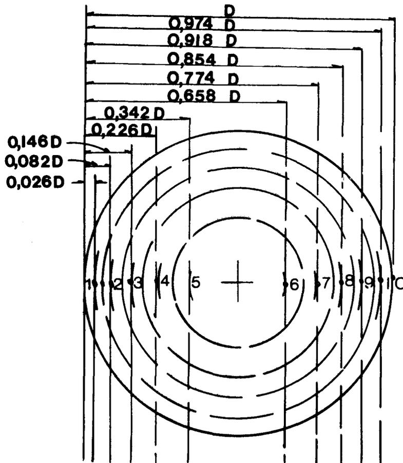
Fig. 5—Equal ring-element areas for velocity measurements
