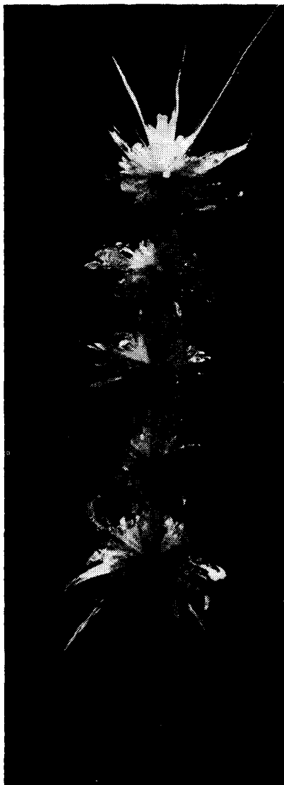
Fig. 3—Cracking round shotholes in PMMA models: 25 mm hole spacing, simultaneous firing
