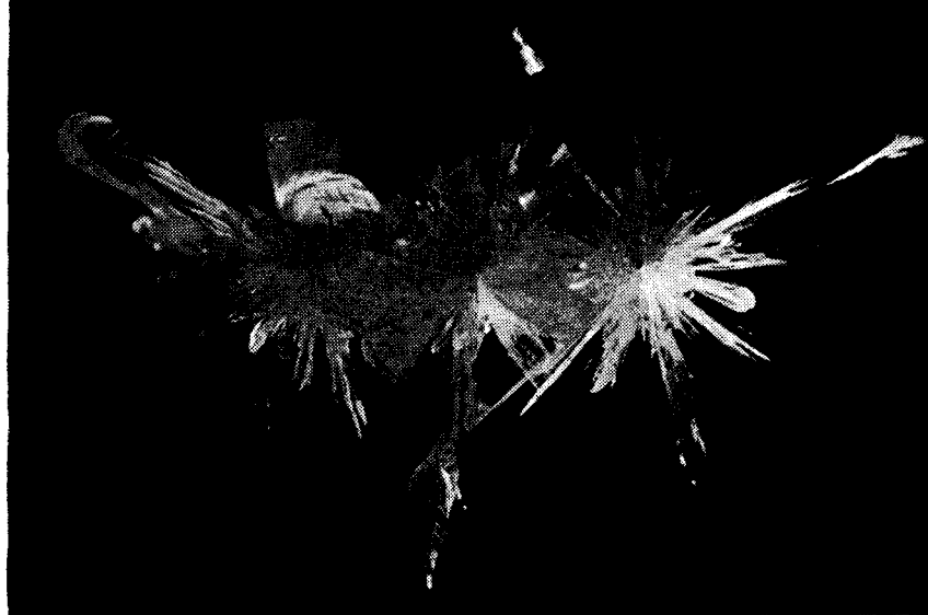
Fig. 4—Cracking round shotholes in PMMA models: 25 mm hole spacing, independent firing
