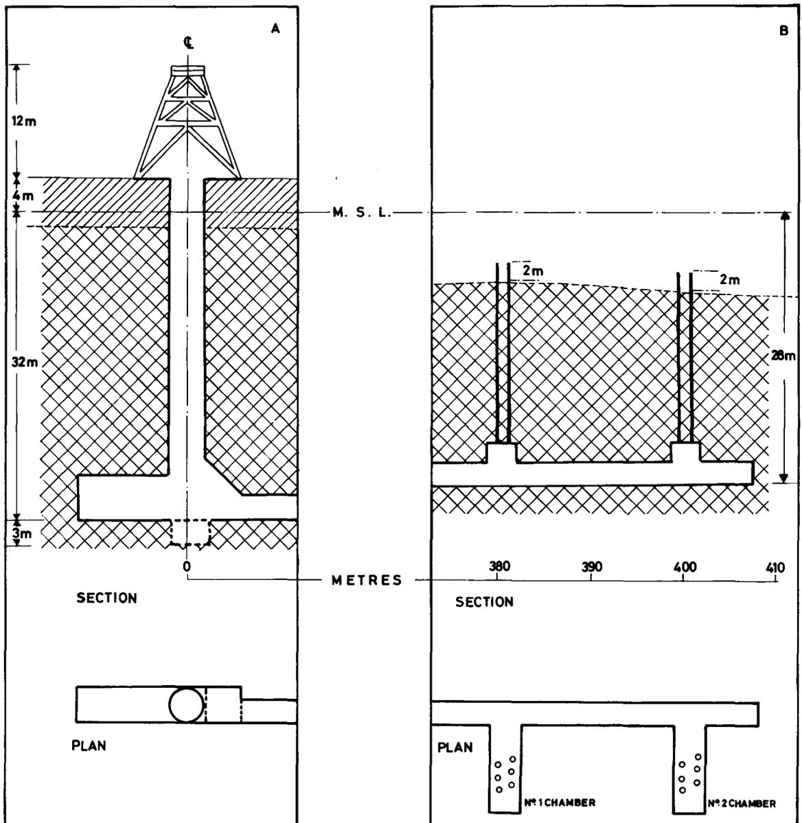
Fig. 5—The sea-water intake system
