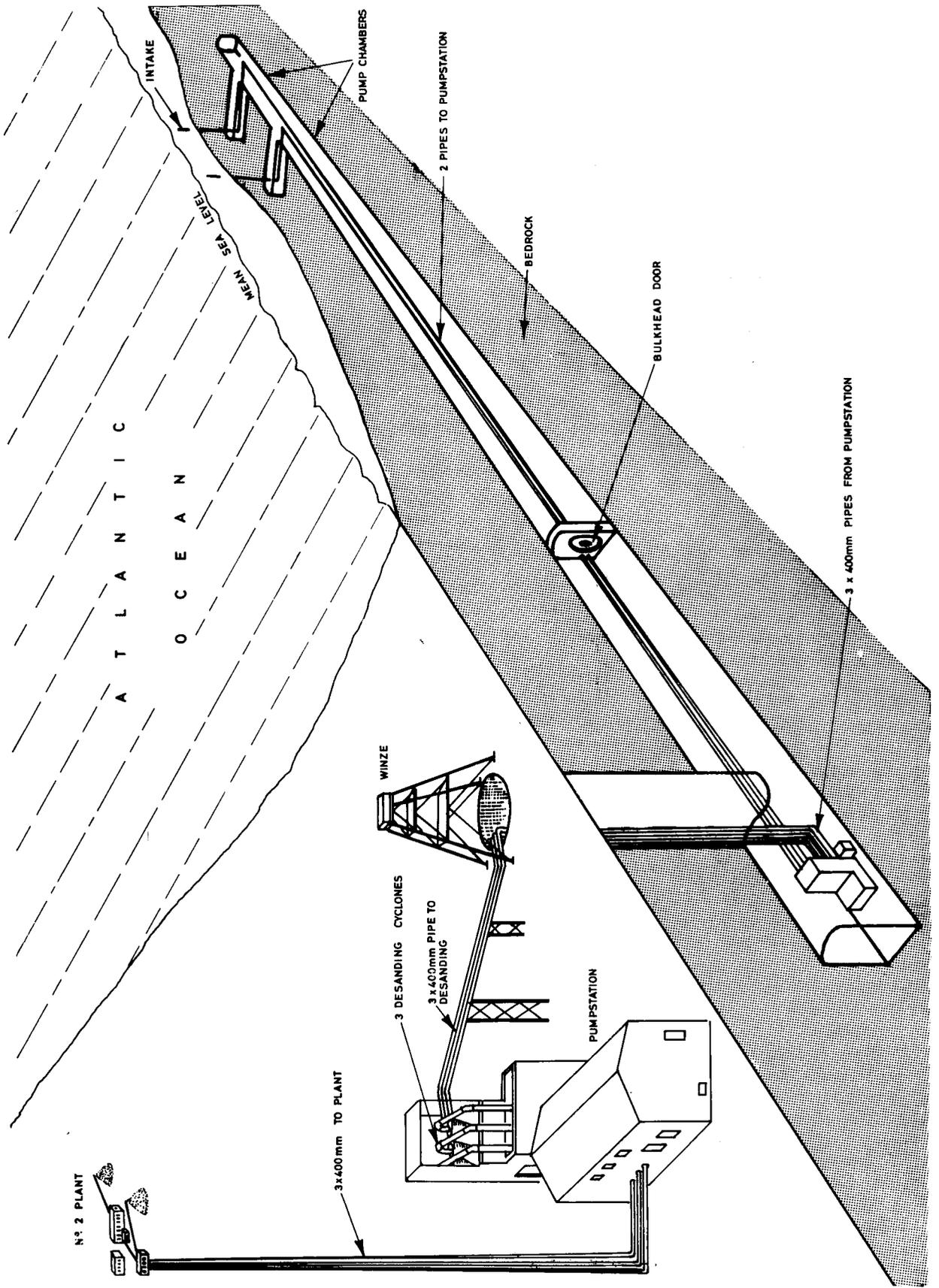
Fig. 7—The pumping configuration
