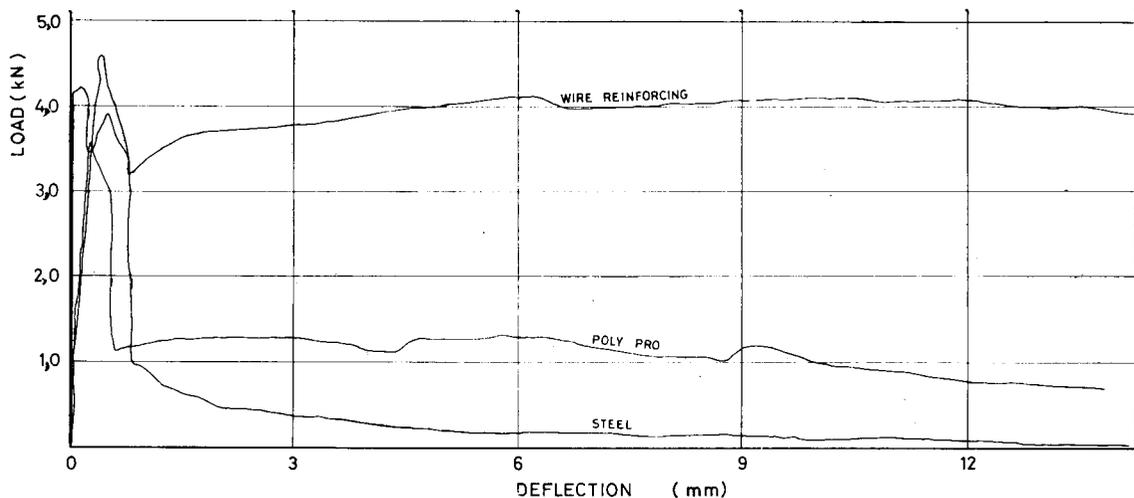
Fig. 3—Comparison between steel fibres (1 per cent), polypropylene fibres (2 per cent), and thick wire reinforcing, no polymer
