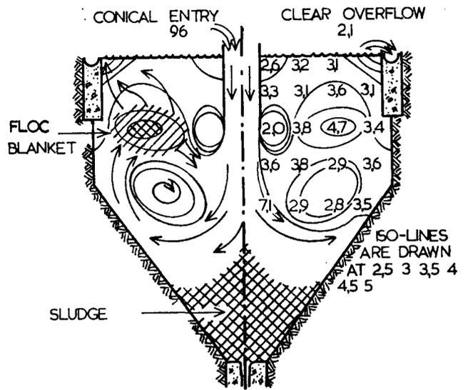
Fig. 4—Flow pattern in a conical settler (the solids analyses are given in p.p.m.)
