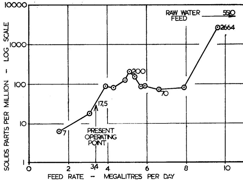
Fig. 6—Feed rate to conical settler versus clarity of overflow water
