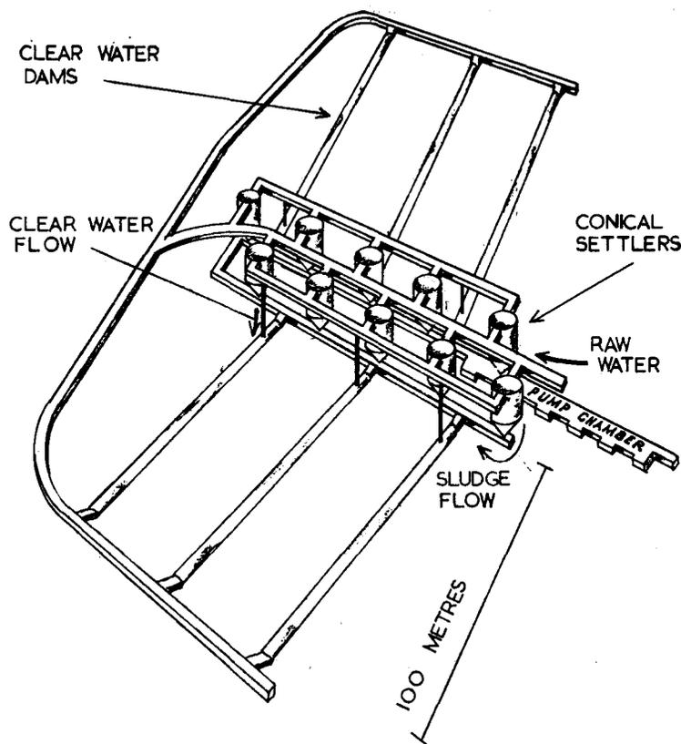
Fig. 7—Layout of new pump chamber, clear water dams, and conical settlers
