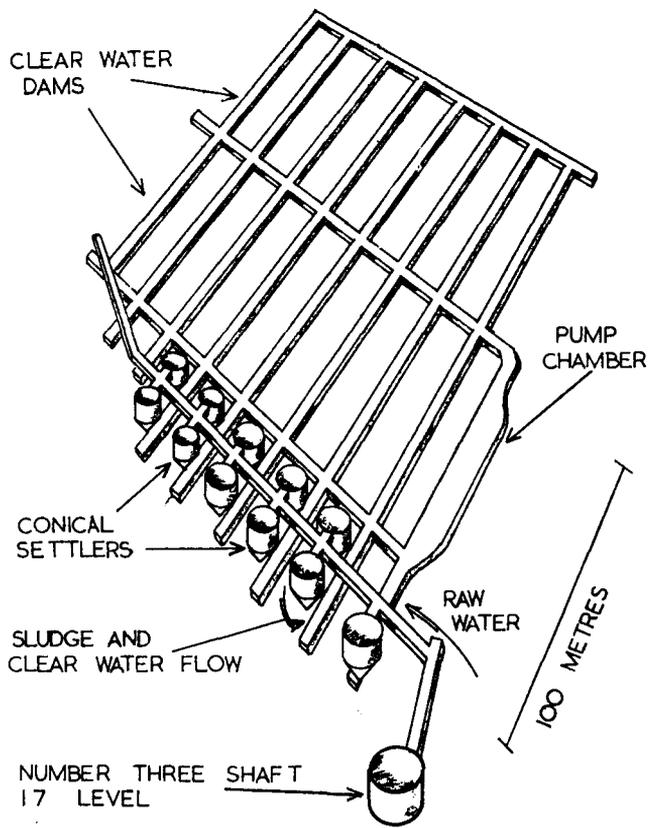
Fig. 2—Isometric view of the pump chamber, clear water dams, and conical settlers
