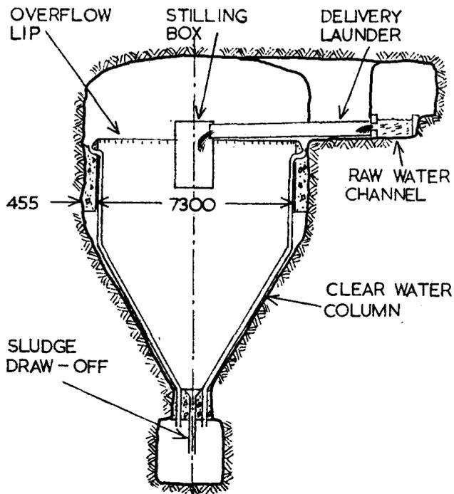
Fig. 3—Cross-section of a conical settler
