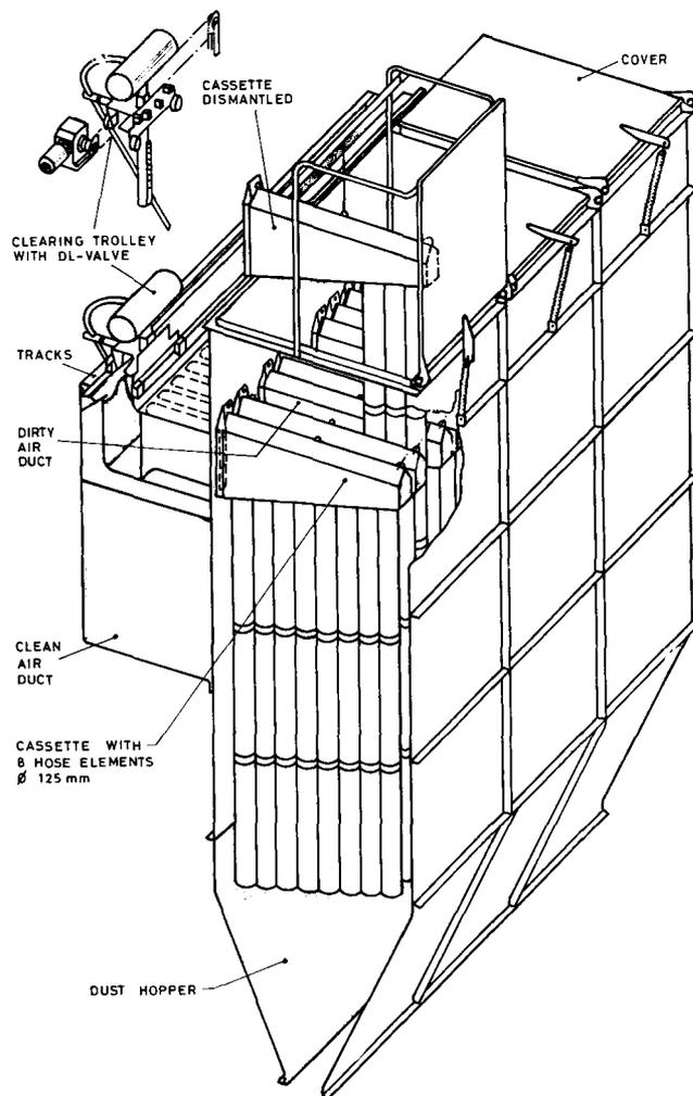
Fig. 2—Detail of filter plant for 6 MV.A open carbide furnace
