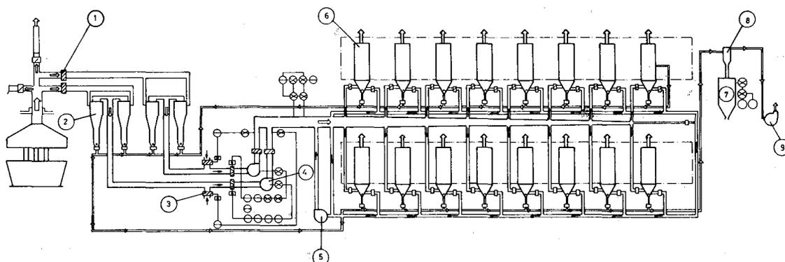
**Fig. 3—Schematic diagram of filter plant for 46,5 MV.A open ferrosilicon furnace**
