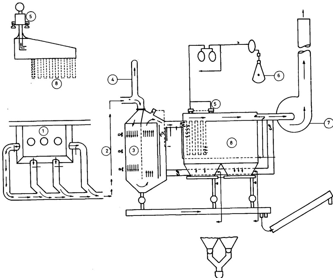
Fig. 1—Schematic diagram of filter plant for 6 MV.A open carbide furnace
