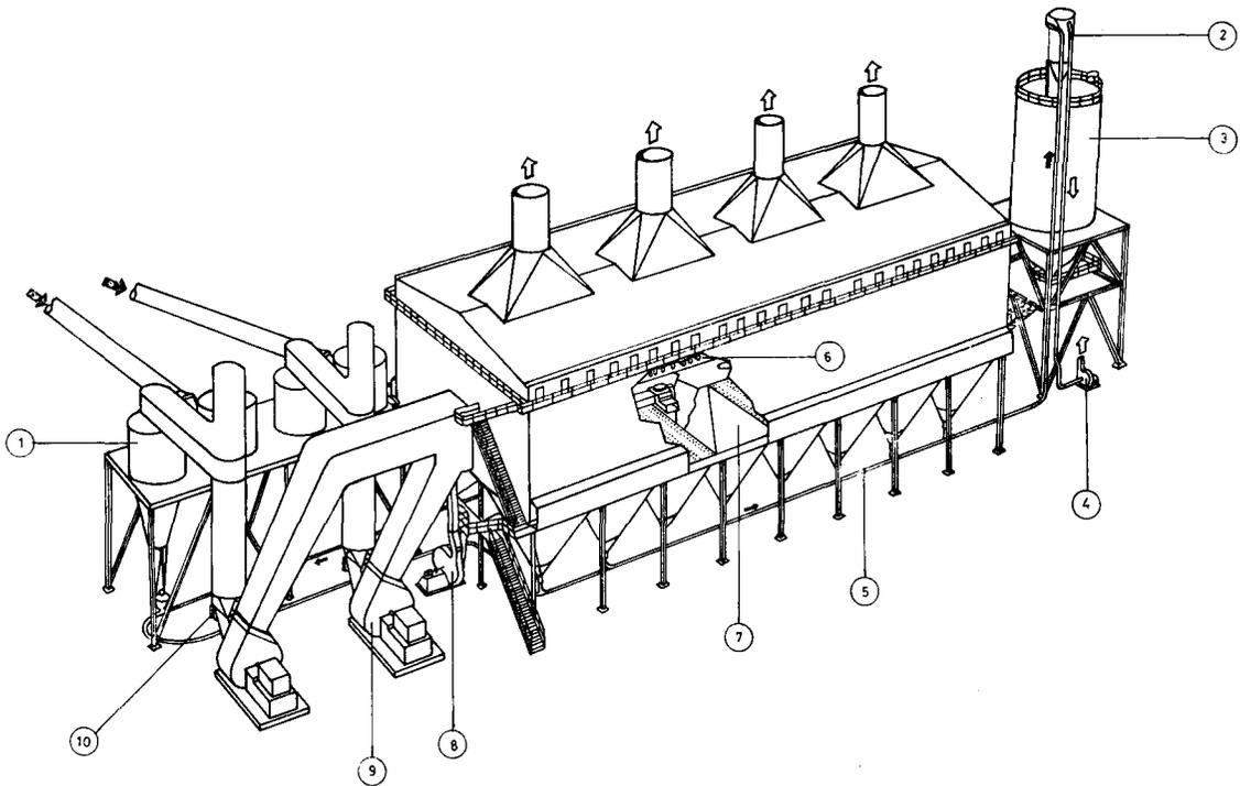
Fig. 4—Filter plant for 6 MV.A open carbide furnace
