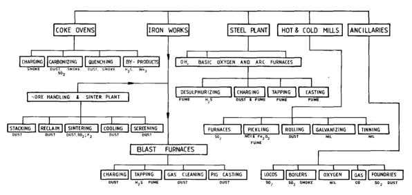
Fig. 4-Possible sources of air pollution in an integrated steelworks
