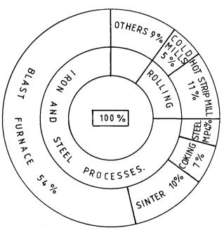
Fig. 3-Energy required for steelmaking
