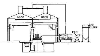
Fig. 14—Combined furnace extraction with full roof extraction
