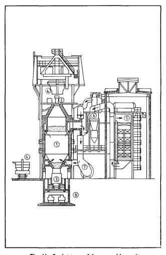
Fig. 11—Soviet type of dry quenching unit
