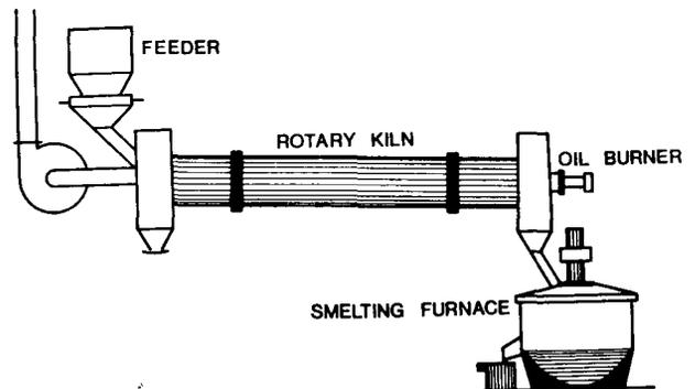
Fig. 3—200 kW pilot furnace and rotary kiln
