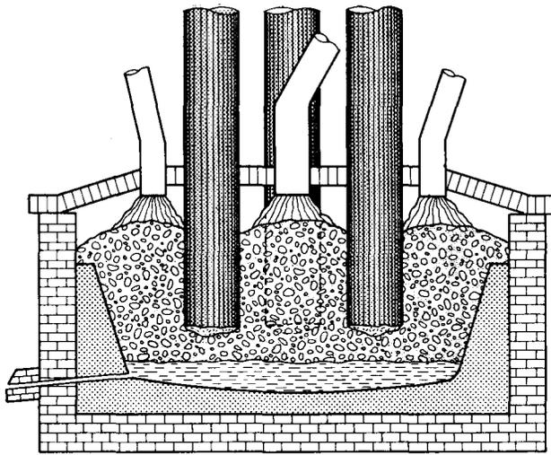
Fig. 4—Three-phase industrial furnace
