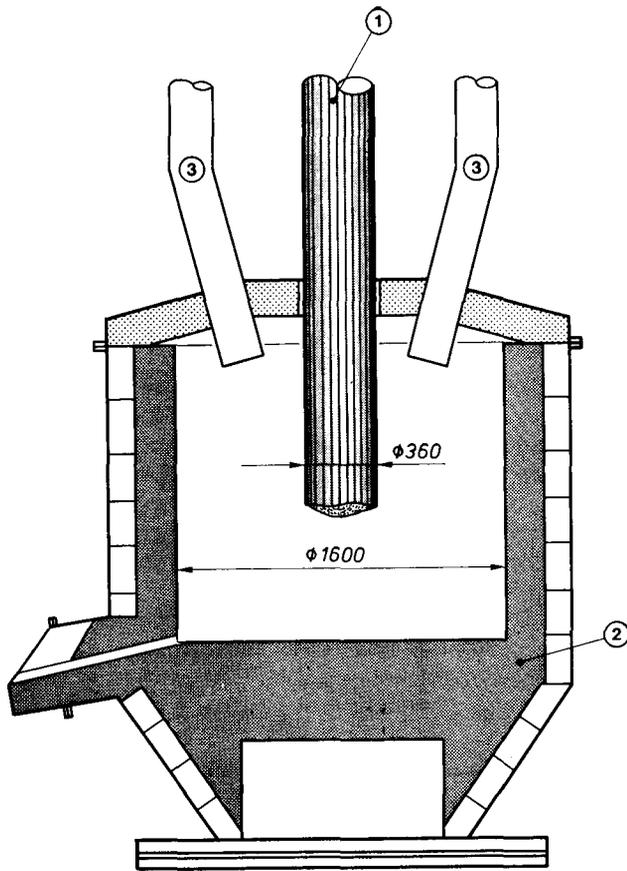
Fig. 2—500 kW pilot furnace
