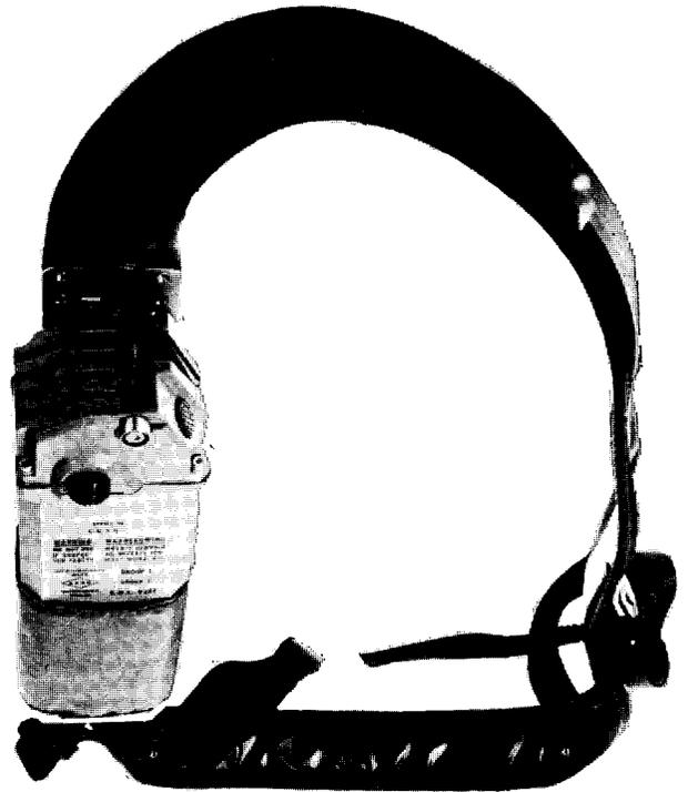
**The SC 100 Substrata Communicator is mainly used for voice communication in mines. This highly sensitive portable unit permits speech through up to half a kilometre of solid rock. As a technological breakthrough by a Chamber of Mines research team, the Communicator is of particular significance in emergency situations, permitting Proto teams to maintain efficient contact under extreme conditions.**
