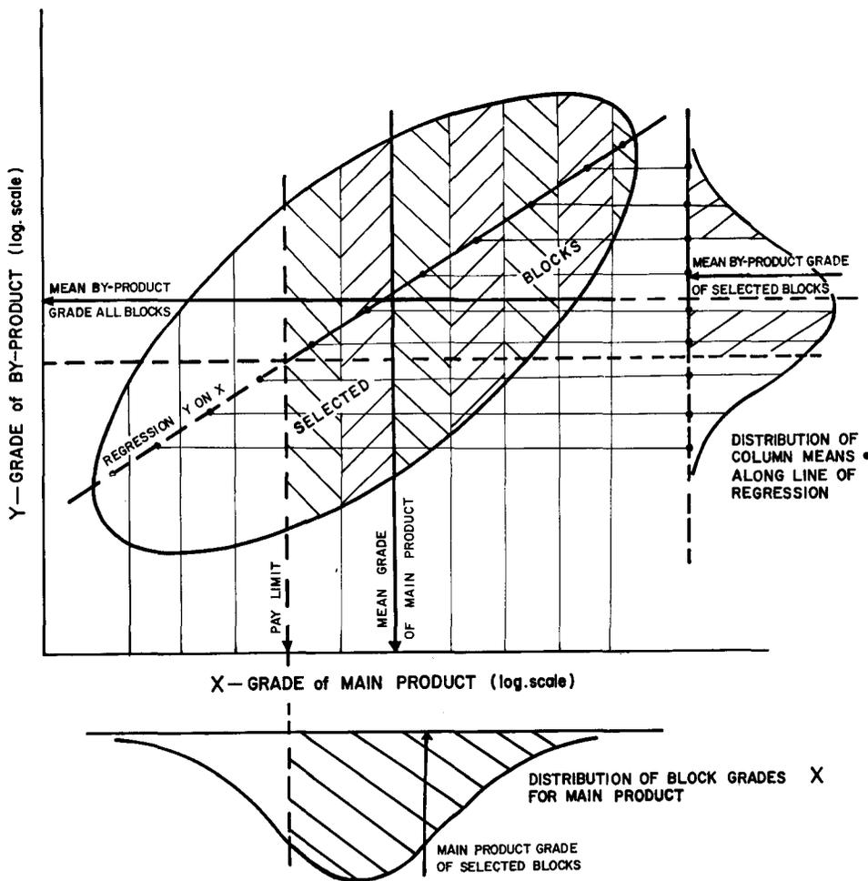
Fig. 4—Lognormal model for estimating tonnage and grades of ore selected for mining on main product pay limit
