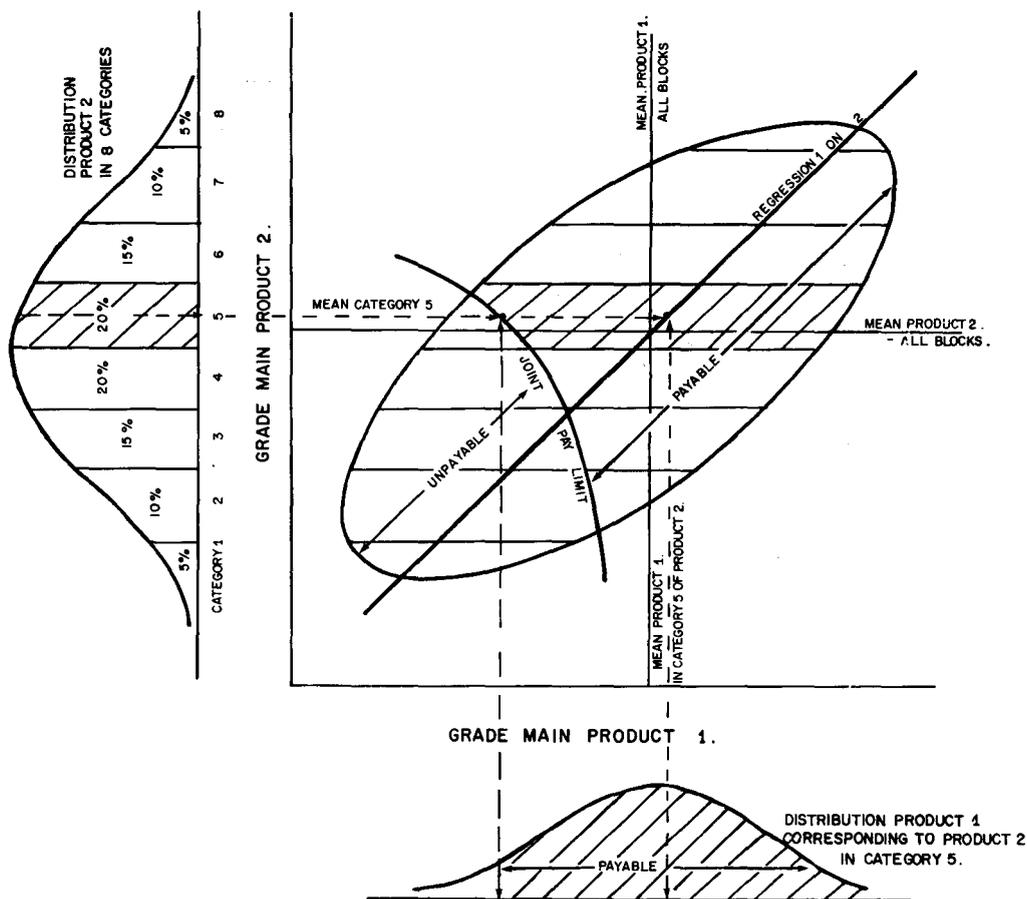
Fig. 5—Bi-variate lognormal model for mining selectively to a joint pay limit based on two main products
