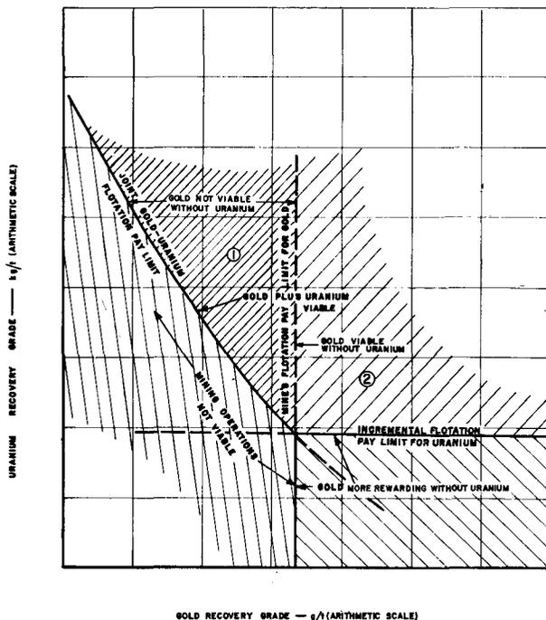
Fig. 3—Illustrating the nature of a joint gold-uranium flotation pay limit for a potential new mine
