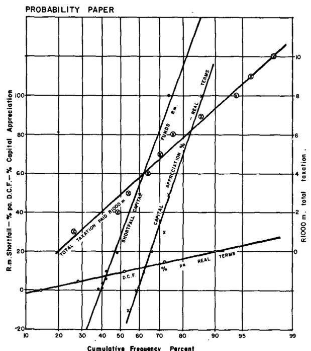
Fig. 1—Normal frequency distributions for some output variables from a risk analysis for a new gold mine based on 50 iterations
